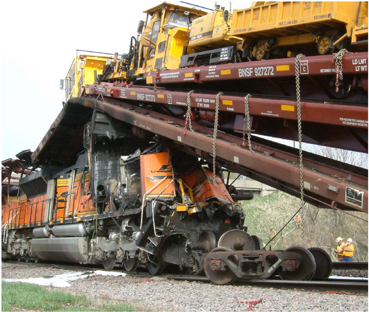
Exhibit 13-Photo Showing Bogie Assembly from BNSF 927022 in Front of BNSF 9159
