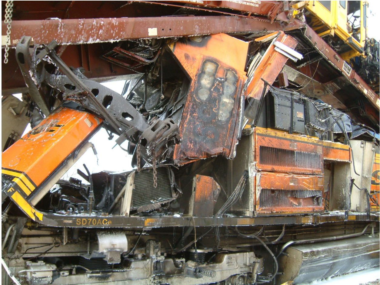
Exhibit 12-Photo Showing Bogie Assembly from BNSF 927022 On Top of BNSF 9159's Short Hood
