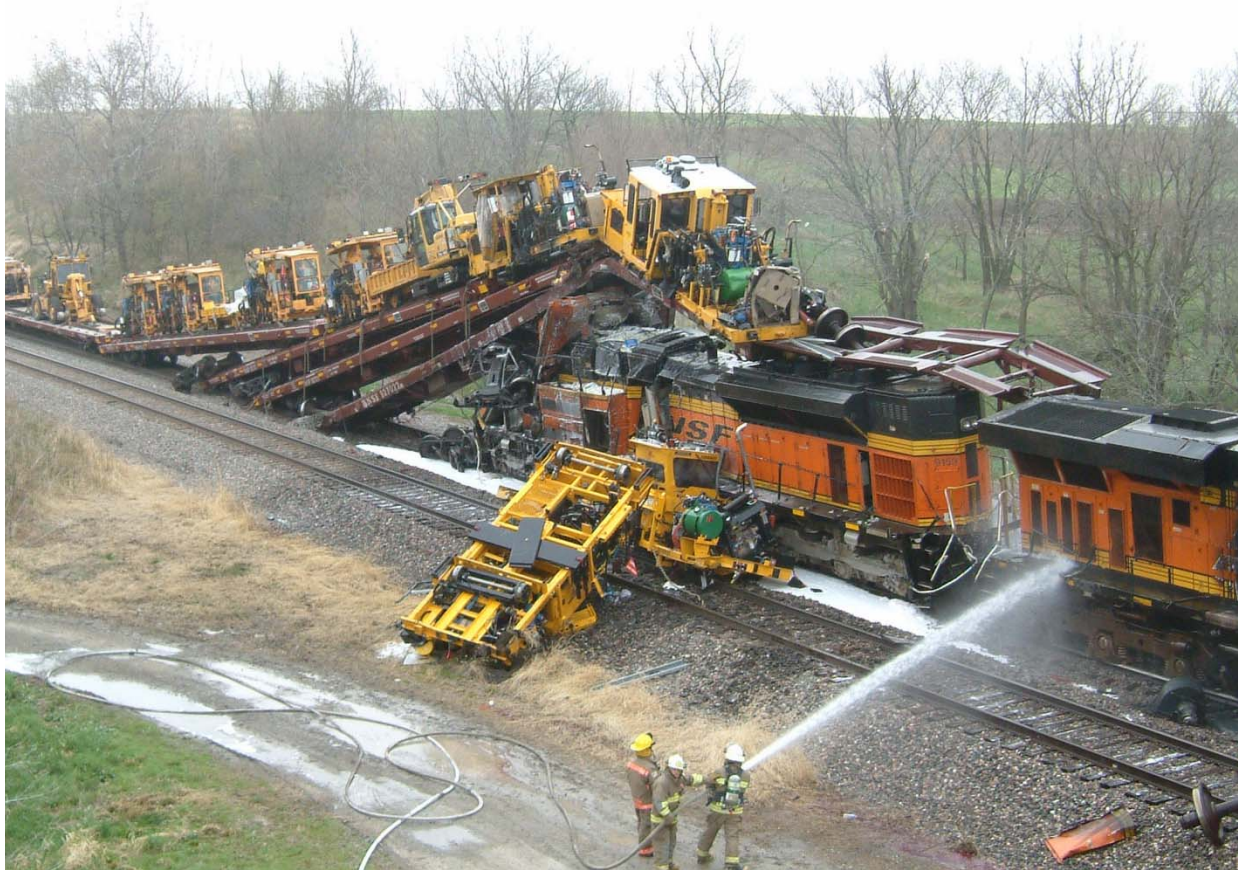
Exhibit 11- Photo Showing BNSF 927022 Overriding BNSF 9159 with Loading Ramp Extended Overtop of Locomotive
