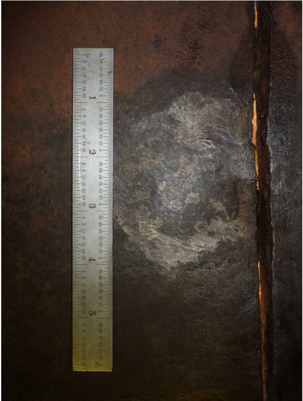
Corrosion repair pad welding near tank crack, August 31, 2016
