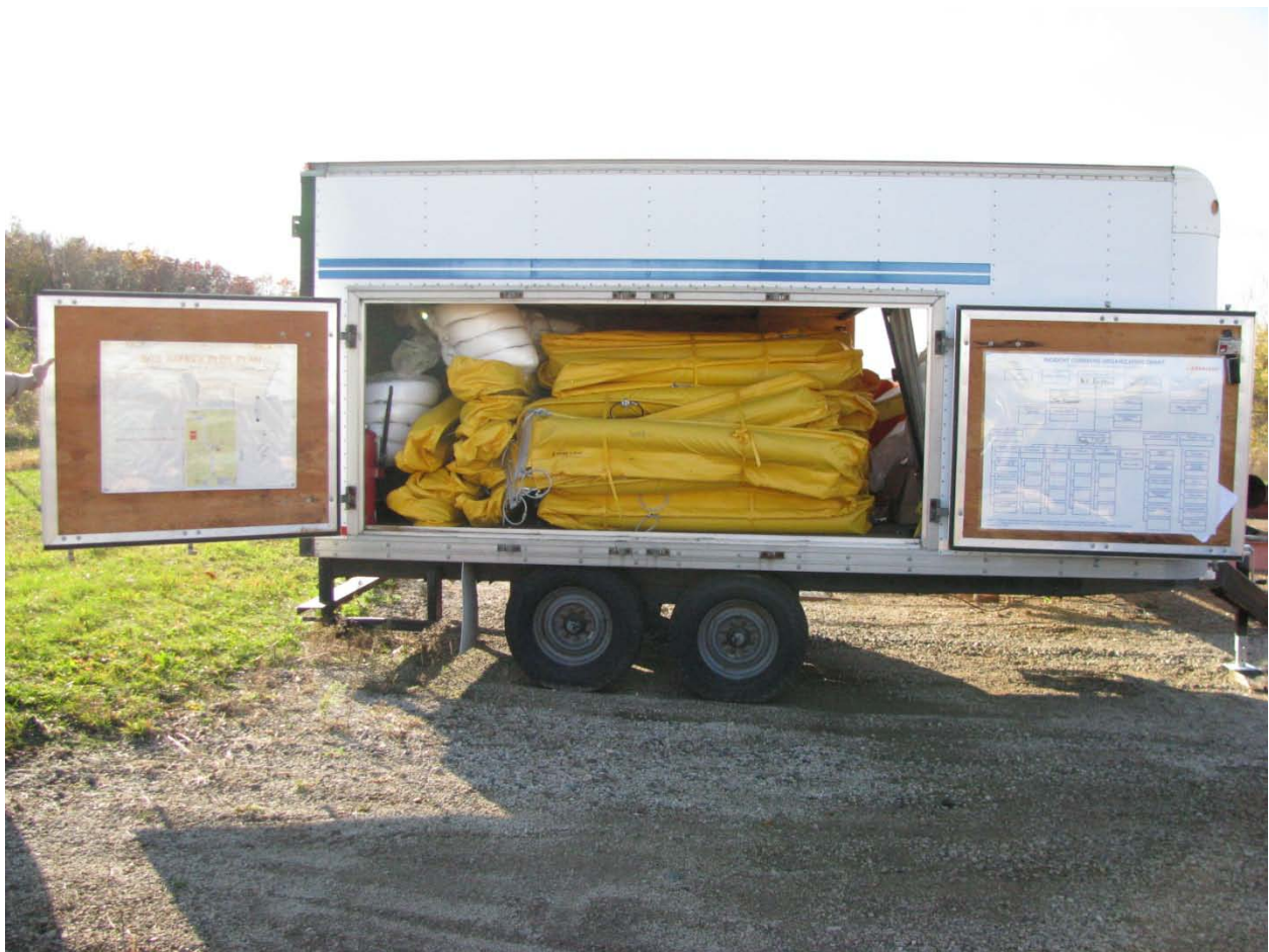
Figure 20. Enbridge PLM emergency response trailer containing the company's Tier 1 oil containment equipment, October 17, 2010.
