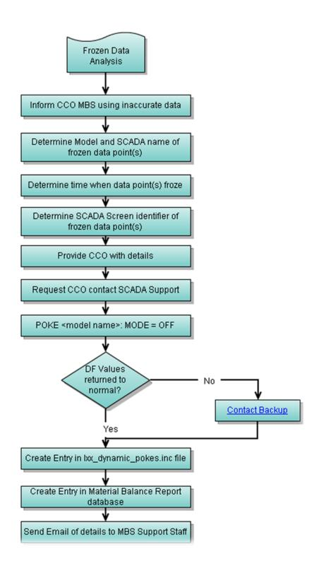
3) Using the flow chart to respond to a field maintenance notification (Flow meter to be taken out of service for repairs).
