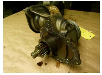
Crankshaft to Camshaft Timing The crankshaft to camshaft timing was verified by the alignment of the gear's timing marks.
