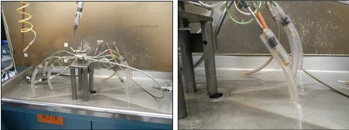
Figure 3: One O-ring fuel manifold and nozzle flow test.
