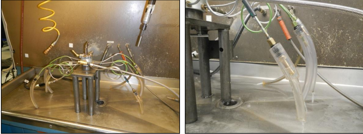
Figure 2: Two O-ring fuel manifold and nozzle flow test.
