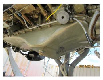
Oil Filter Condition: The oil filter was undamaged and safety wired. The filter was not removed during the inspection as designated by the NTSB.
