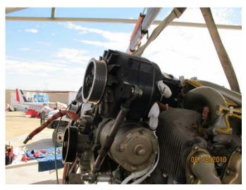
Accessory Gears Condition: The crankshaft was rotated by hand and continuity was obtained from the accessory gears, forward camshaft drive gear and starter drive pulley.
