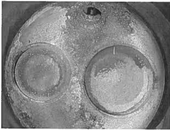
Normal Combustion Chamber. Exhaust valve has reddish combustion deposit in center with dark outer edge. Intake valve has light brown combustion deposits. Combustion chamber has light brown deposits.
