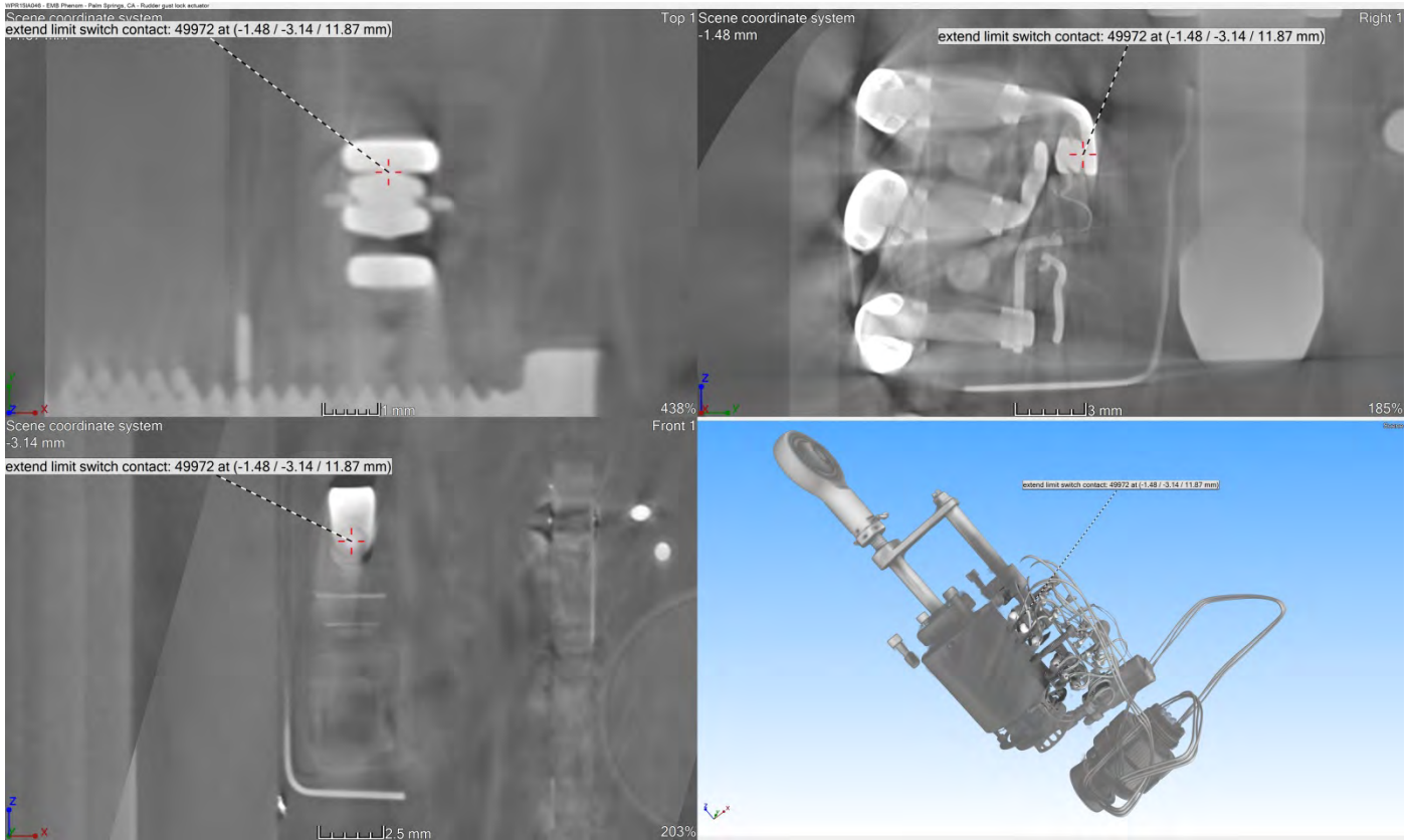
Figure 8 Rudder gust lock actuator – microfocus – extend limit switch contact point
