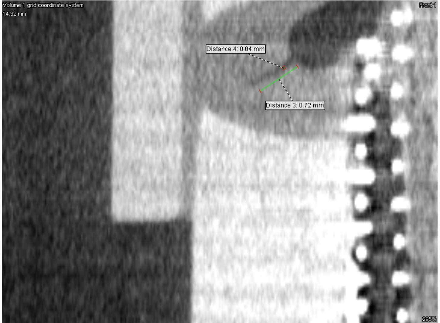
Figure 19 Frontal view – Return Filter (section 458-468) – Close up view of crack in epoxy material (not shown in previous figures), measuring 0.72 mm long and 0.04 mm wide
