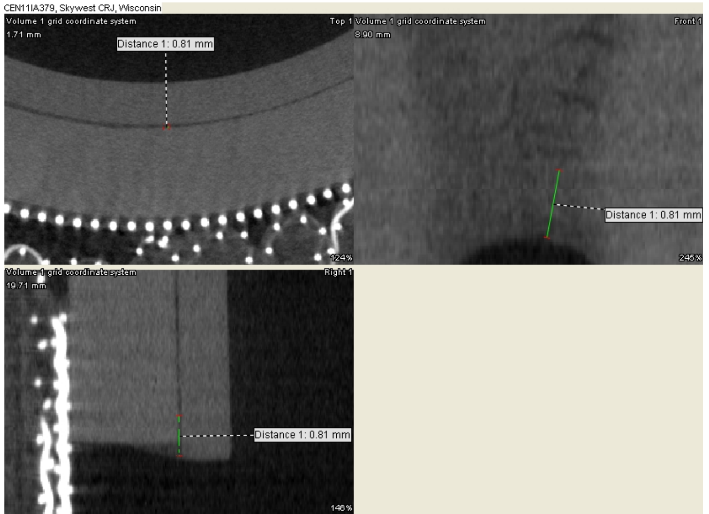
Figure 18 Multiple views – Return Filter (section 458-468) – Views showing the location of the network of cracks in the epoxy material (shown in figure 17)
