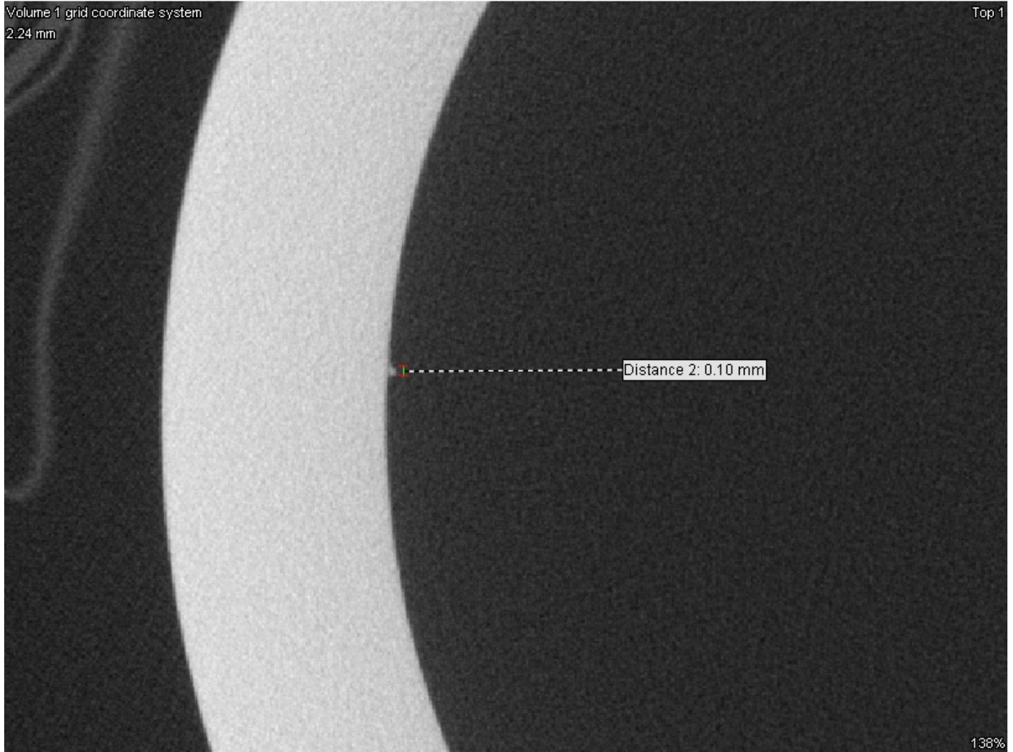
Figure 8 Axial Cross Section – Pressure Filter (section 514-518) – Particle measuring 0.10 mm x 0.13 mm on inside surface of inner support core
