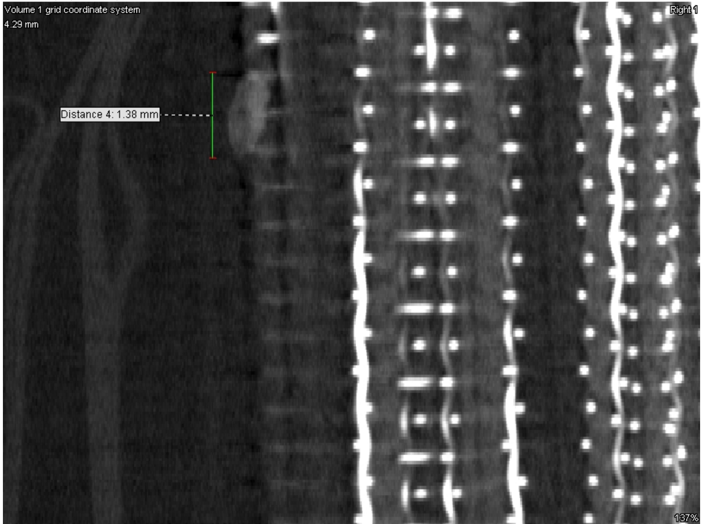
Figure 6 Right Cross Section – Pressure Filter (section 494-504) – Low density particle (shown in figure 5) measuring 0.79 mm x 1.38 mm, on the outer stainless steel mesh
