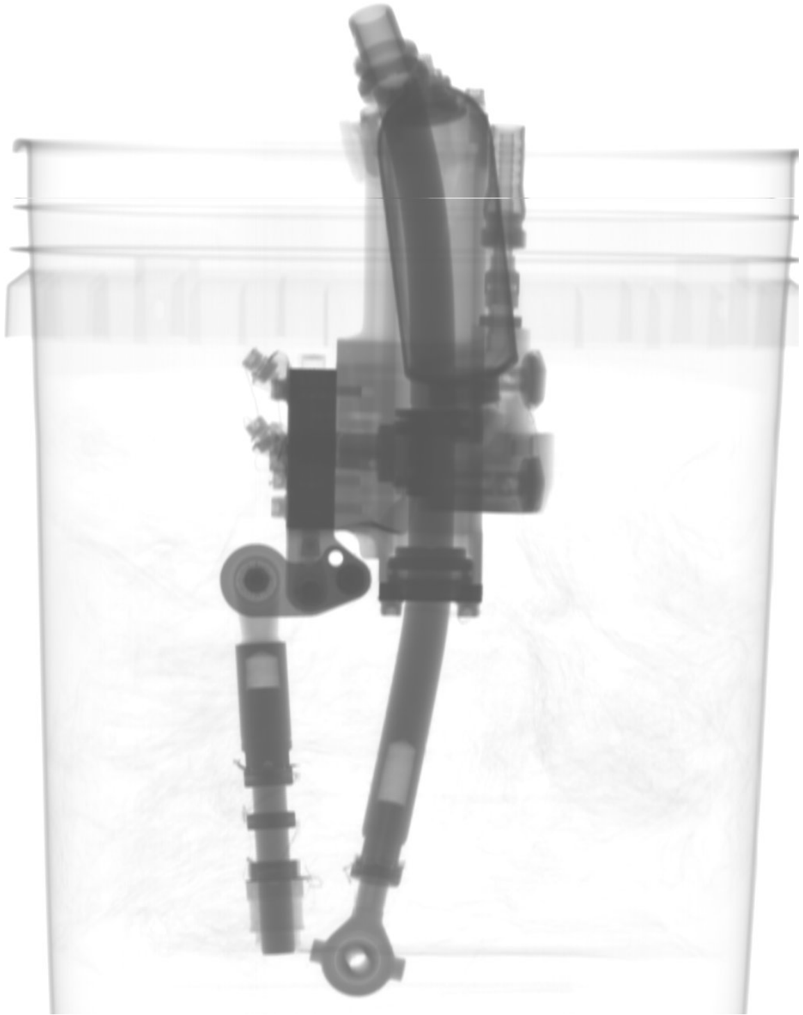
Figure 4 Digital Radiograph – Right Lateral Actuator, rotated view
