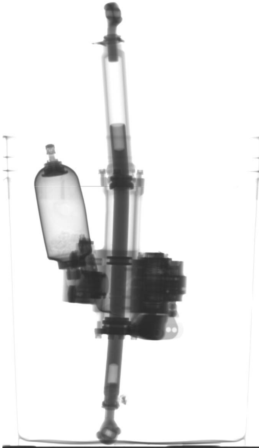
Figure 1 Digital Radiograph – Fore-Aft Actuator
