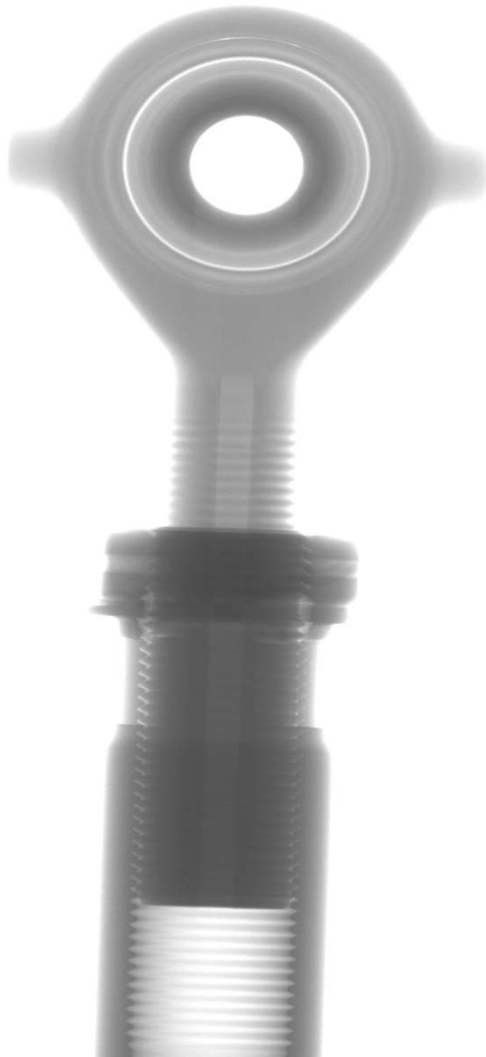
Figure 7 Digital Radiograph – Fore-Aft Actuator Rod End
