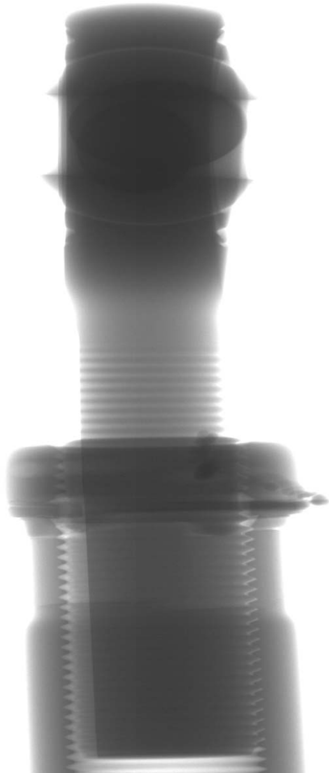
Figure 8 Digital Radiograph – Fore-Aft Actuator Rod End, Rotated View
