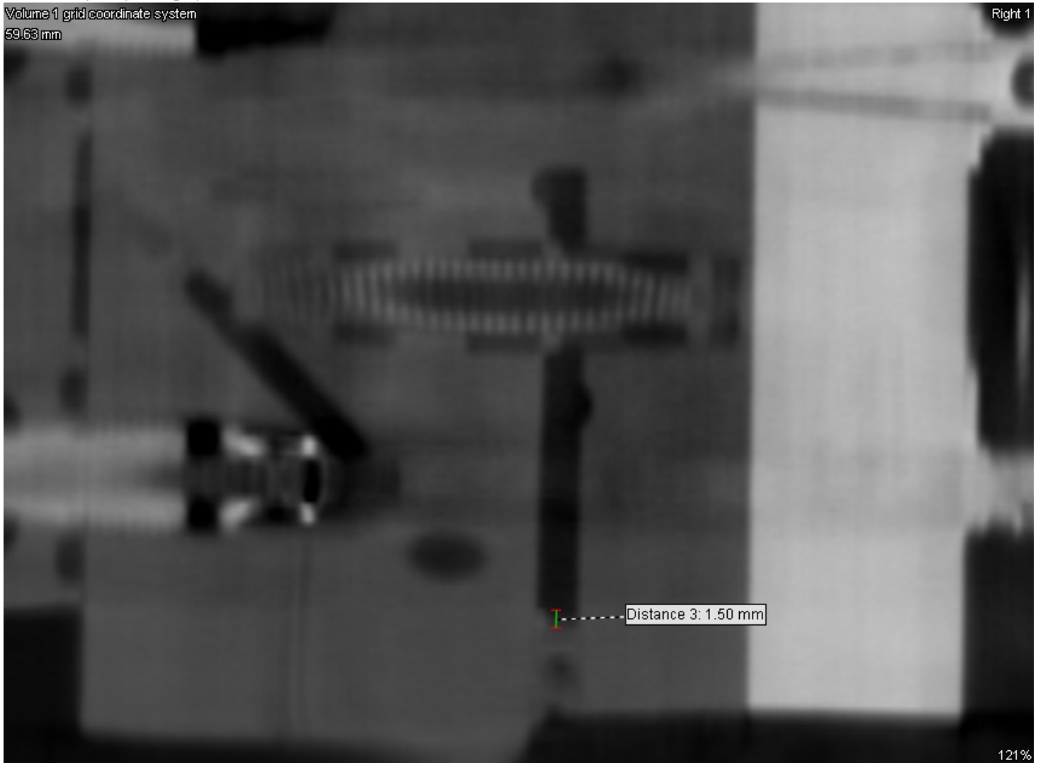
Figure 21 Right cross section – Left Lateral Actuator – Particle 4, measuring 1.50 mm long, at the end of a hydraulic passage
