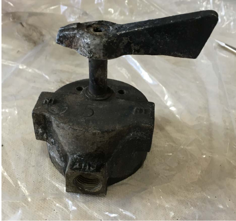
Figure 5: Fuel Selector Valve
