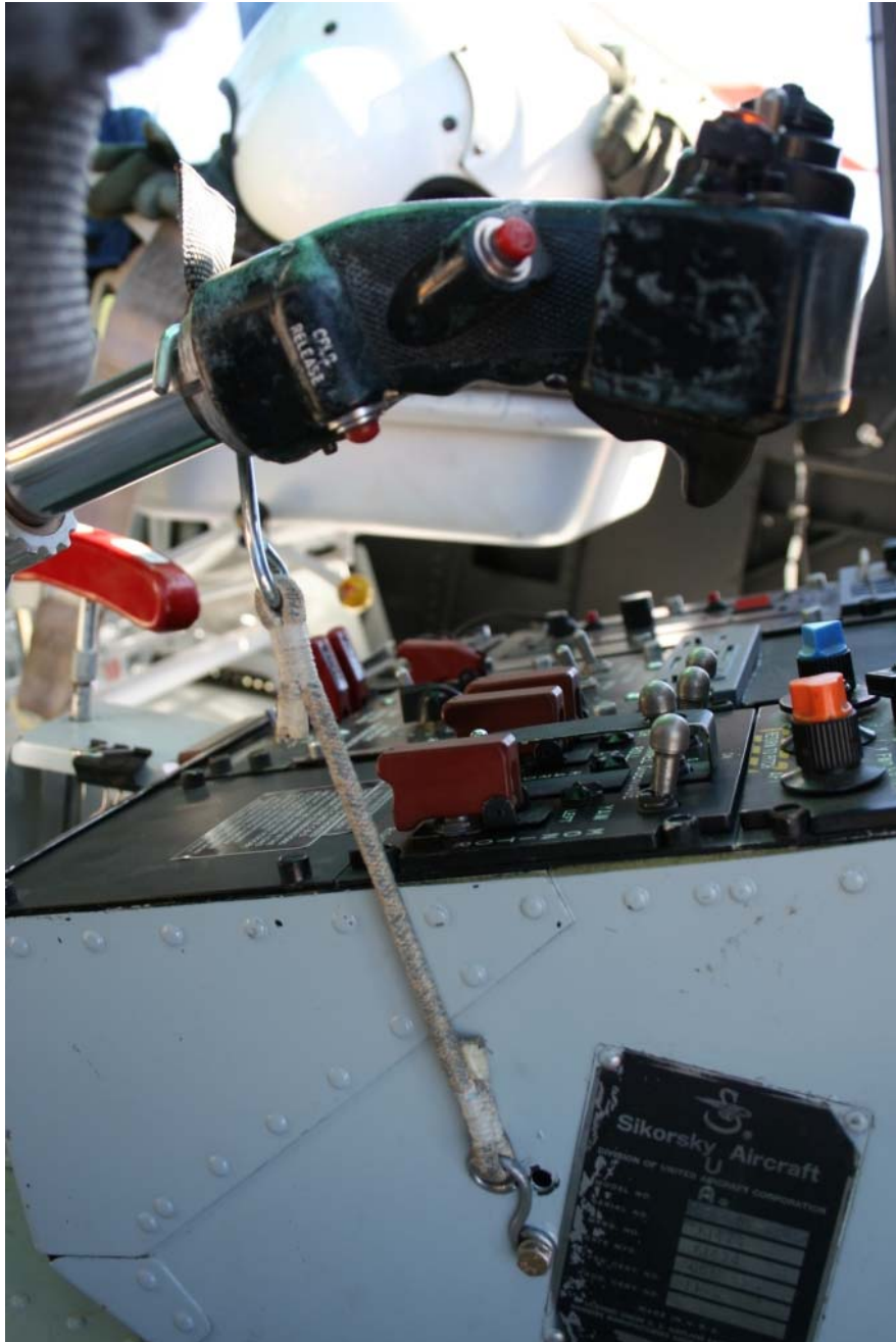
Figure 1: Bungee Installed on N61NH
