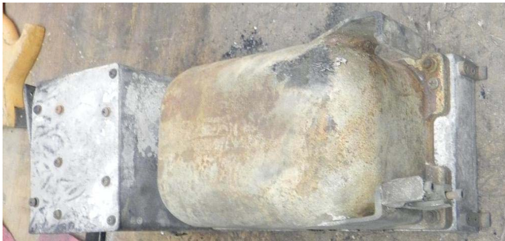
Figure 2. CVR before recovery process.
