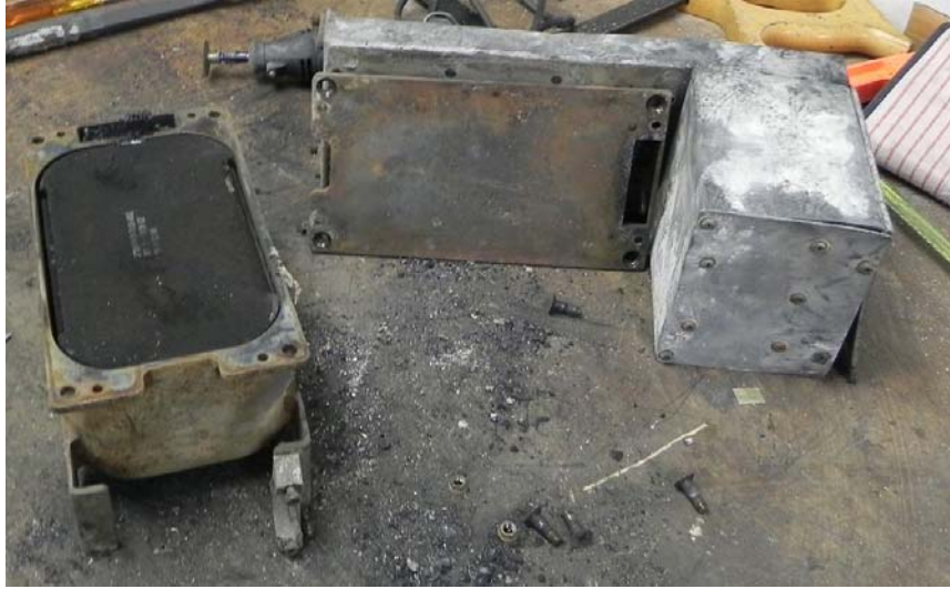
Figure 3. CSMU separated from CVR housing.
