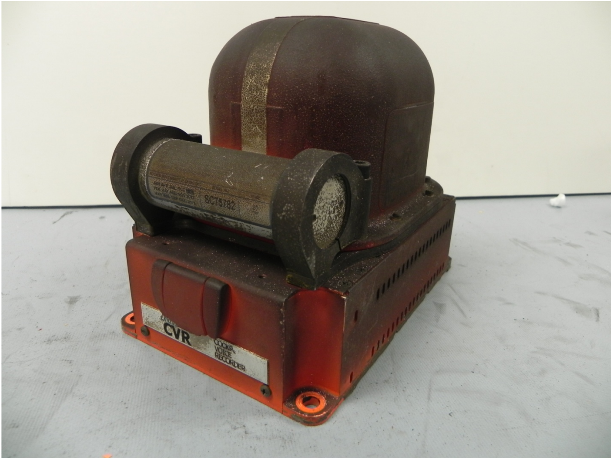
Figure 1. Damaged CVR recovered from G-650 aircraft.
