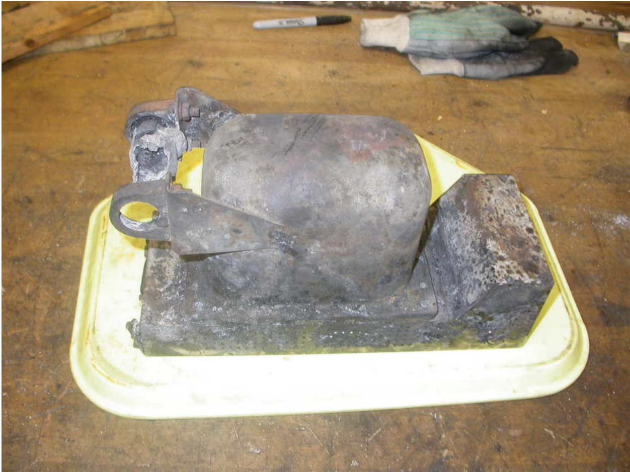
Figure 1. External view of the Universal 1603-02-12 (s/n 1629) showing extensive heat/fire damage.
