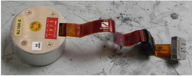
Figure 2. CVR memory device.
