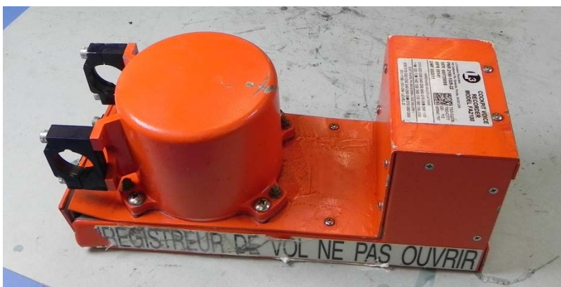
Figure 1. CVR upon arrival at laboratory.
