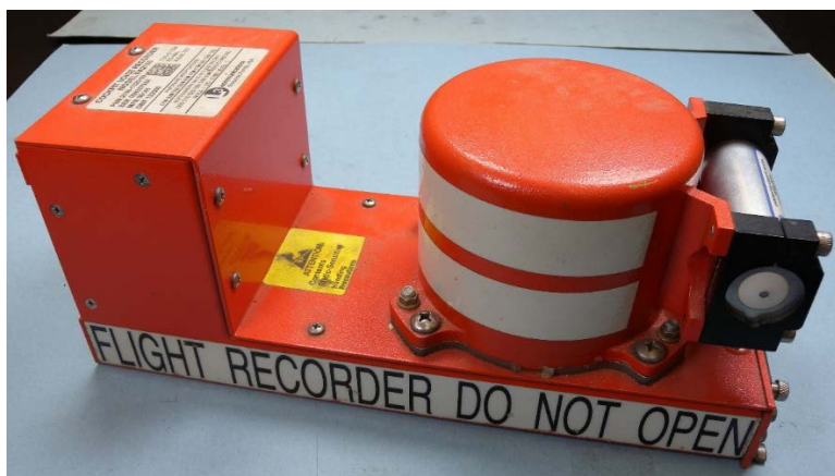
Figure 1. L-3/Fairchild FA2100-1020 CVR recovered from N786TW.
