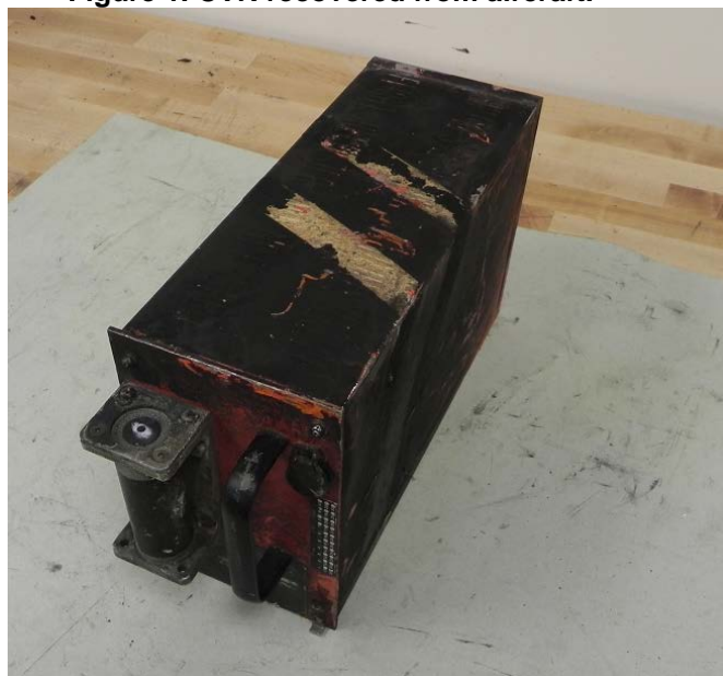
Figure 1. CVR recovered from aircraft.
