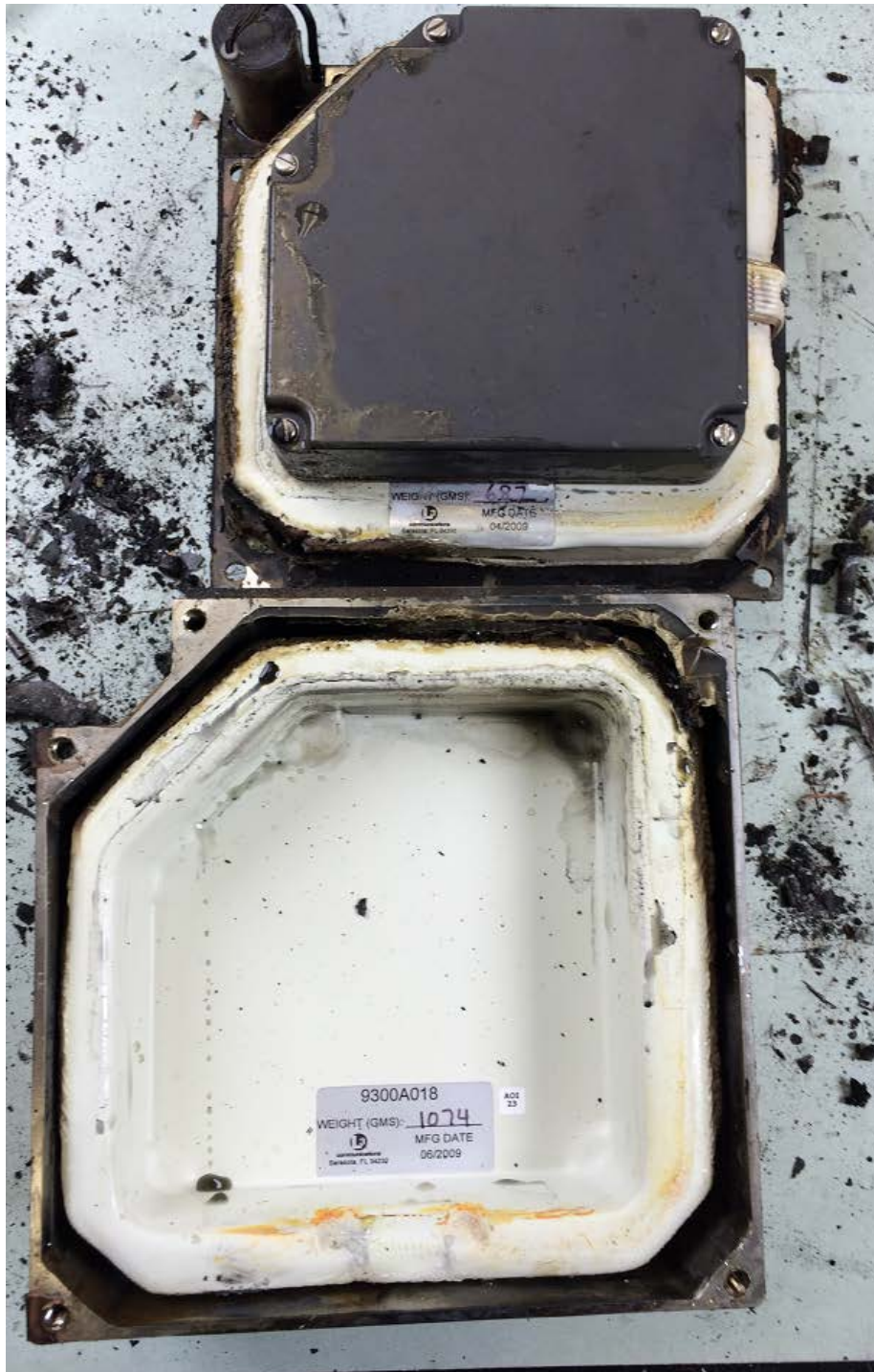
Figure 2. CVR crash-protected case (opened).
