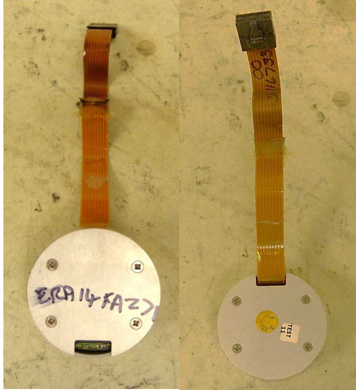
Figure 2. Memory module from the FA2100-1020 (after cable replacement).
