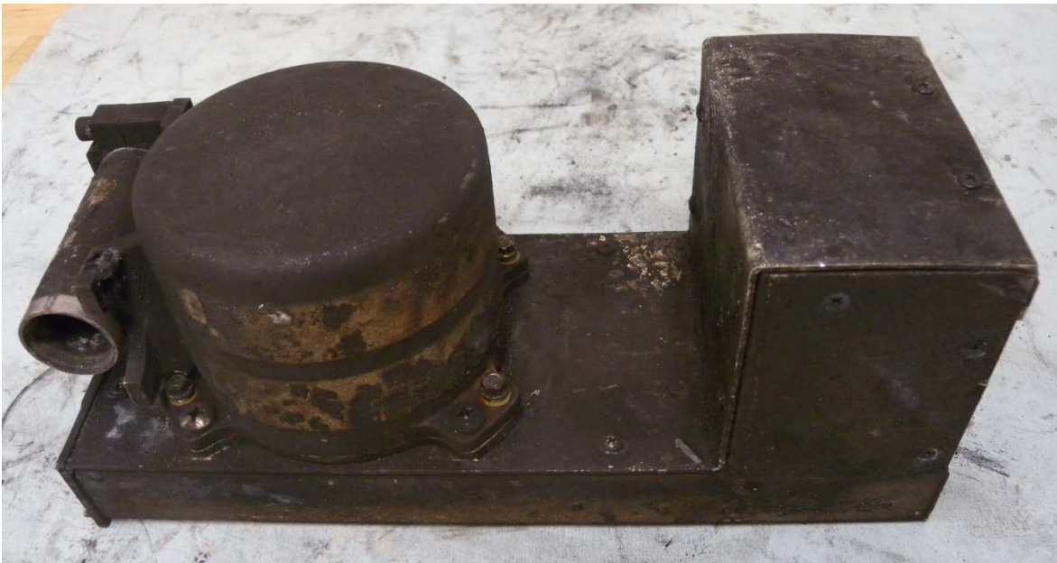
Figure 1. L-3/Fairchild FA2100-1020 CVR recovered from G-IV, N121JM.
