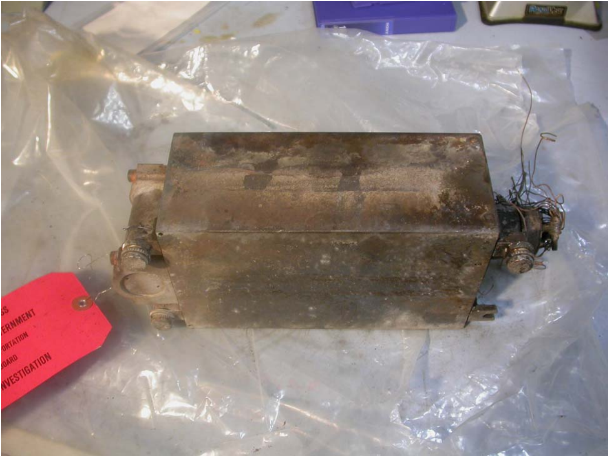
Figure 1 Burned Exterior of Recorder
