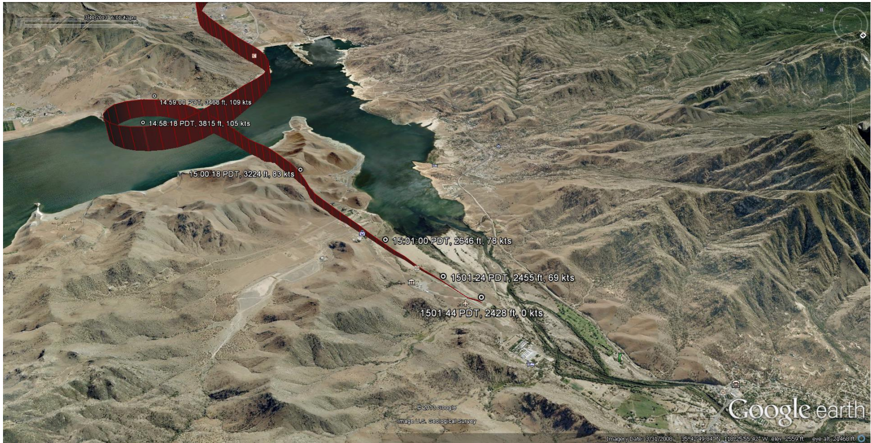
Figure 5. Google Earth overlay showing approach to landing with pressure altitude and indicated airspeed – select points annotated.
