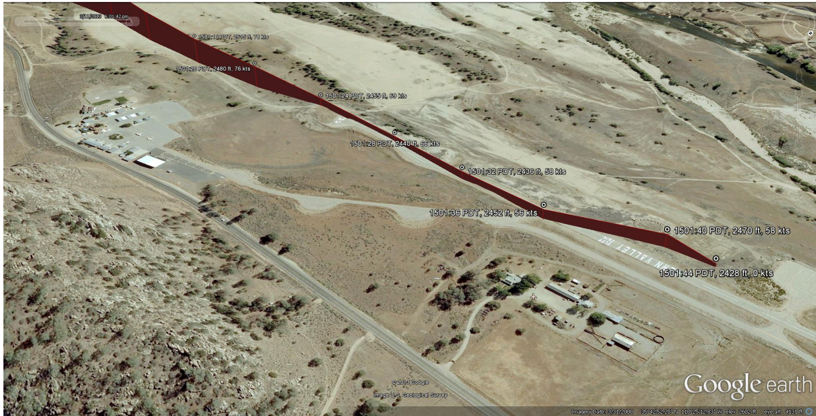
Figure 7. Google Earth overlay showing all points, pressure altitude, and indicated airspeed – short final through runway excursion.
