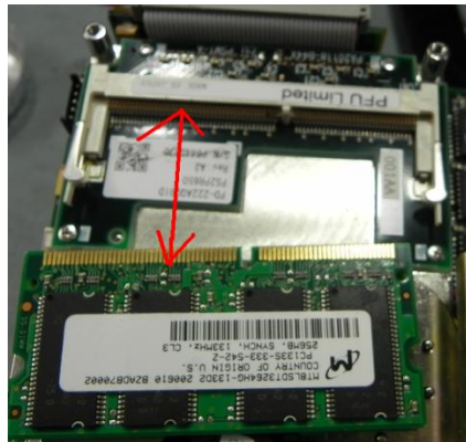
Figure 2. Dislodged internal component (from Sierra Flight Systems IDU Serial Number 201).
