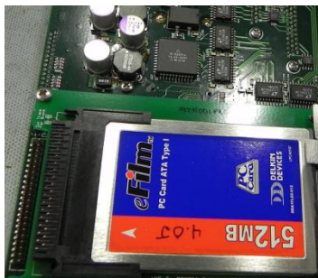
Figure 3. Internal PCMCIA card from Sierra Flight Systems IDU Serial Number 201.
