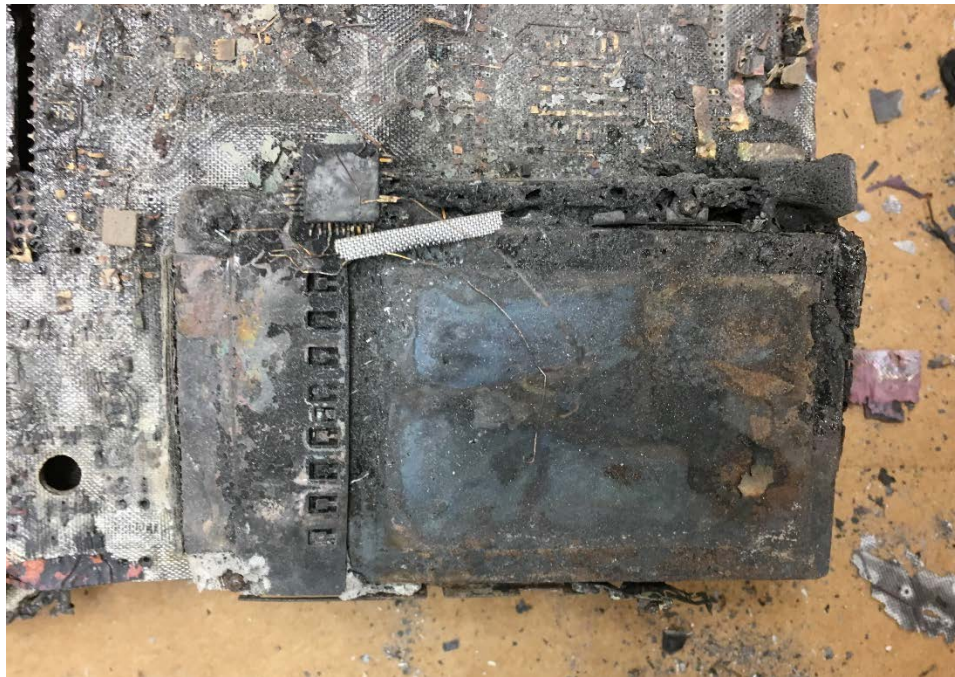
Figure 3. Photo of damaged PCMCIA flash memory card on unit #1
