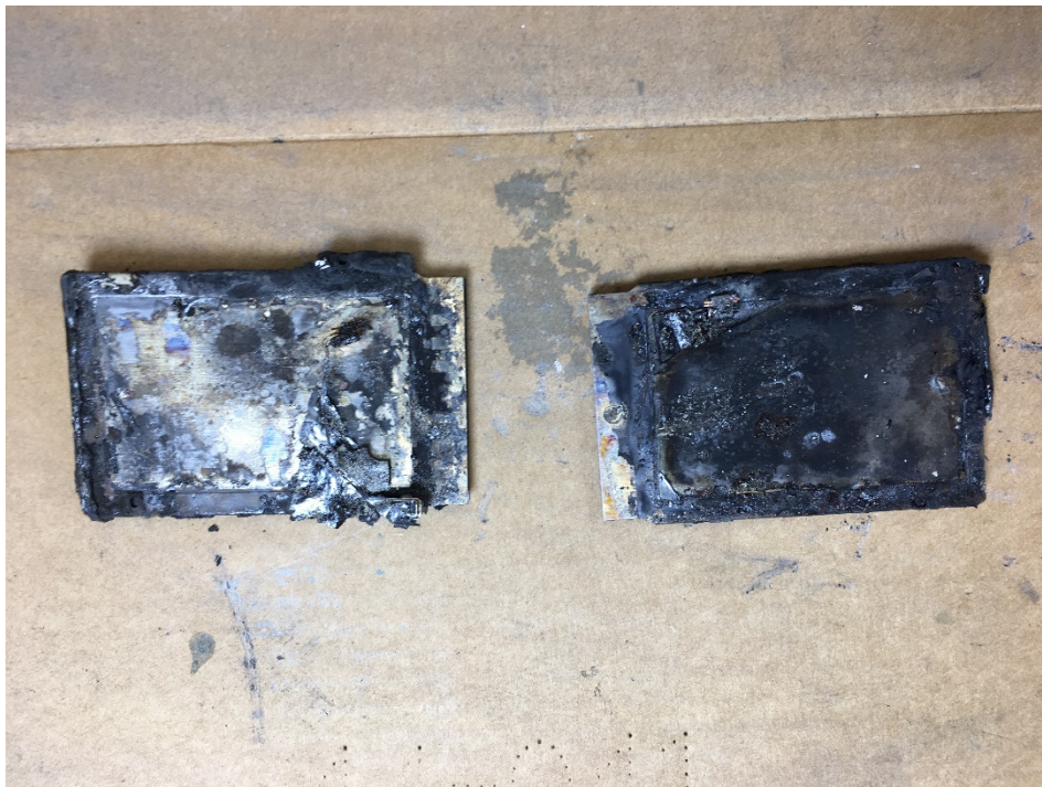
Figure 4. Photo of damaged PCMCIA flash memory card on unit #2
