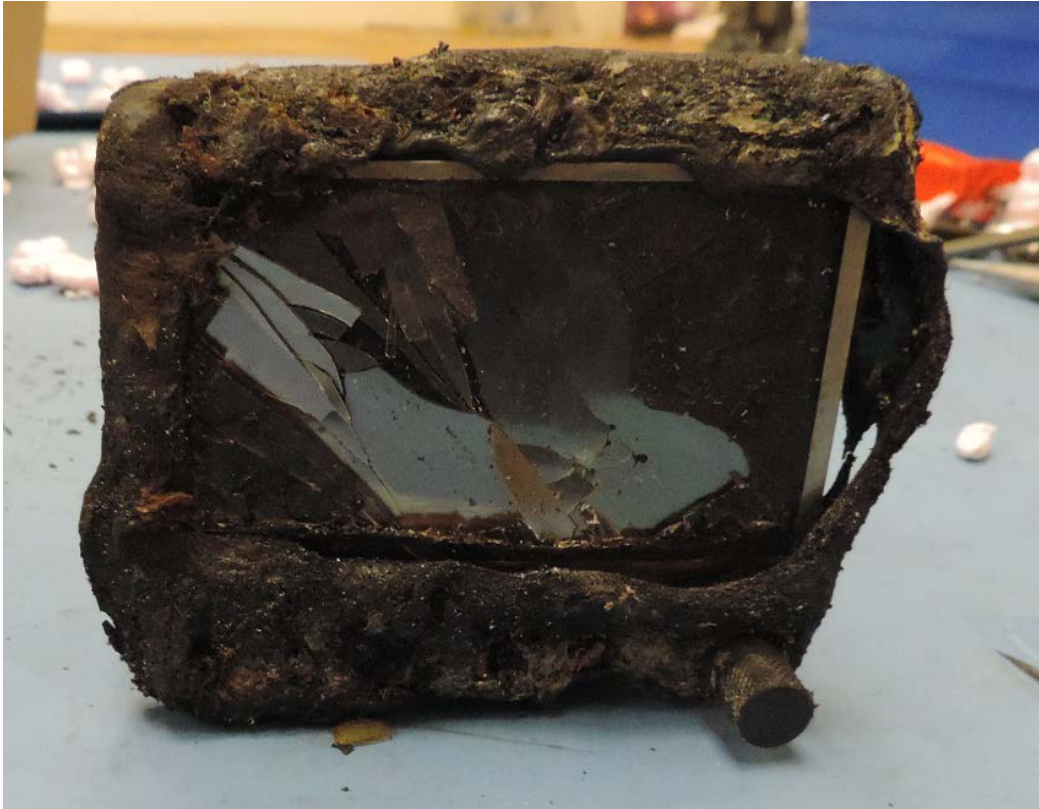
Figure 1. Xtreme-EFIS, after removal from instrument panel.
