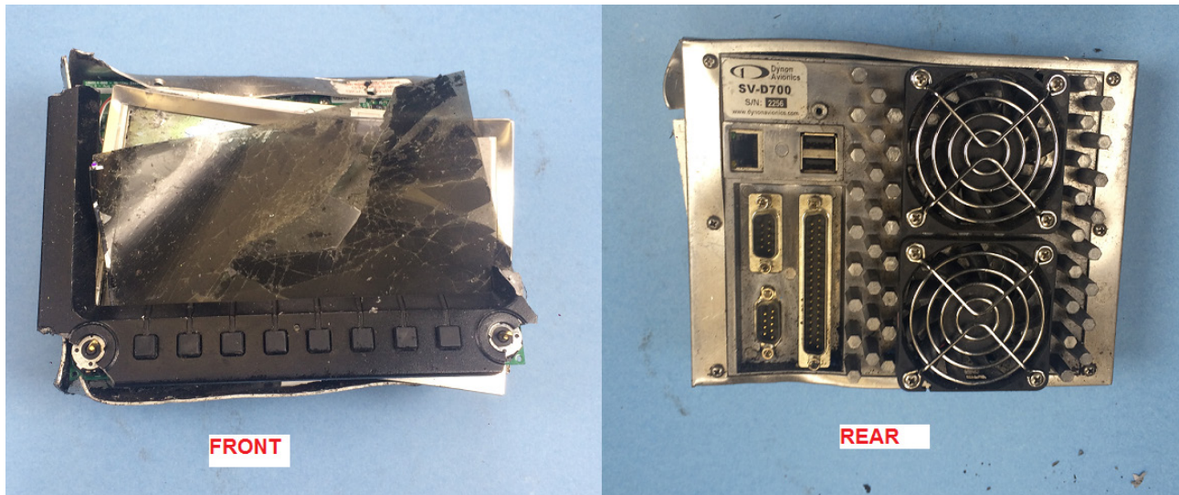
Figure 1. Damaged exterior of Dynon SV-D700.
