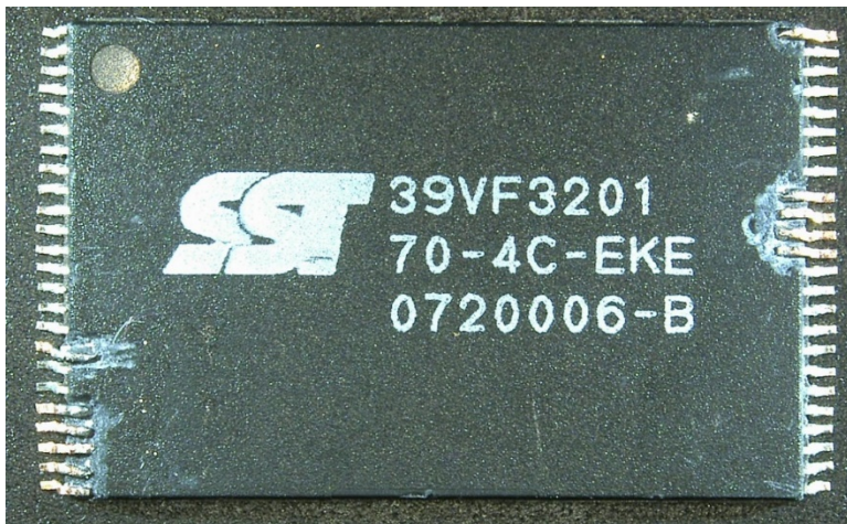
Figure 6. Chip with all connectors repaired.
