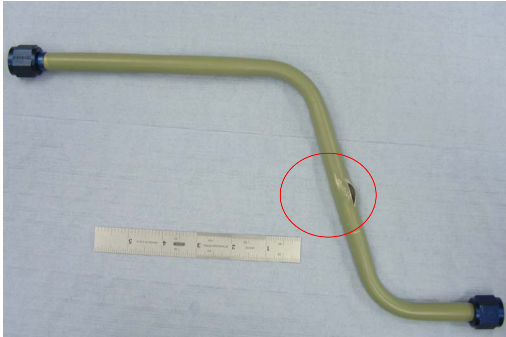
Photo 1 Overall view of the burst 6627002-16 Tube Assembly. Location of burst is circled.
