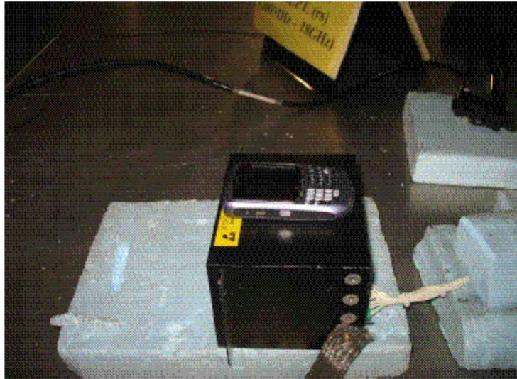
Figure 3-3: Blackberry Placed on PCB Enclosure
