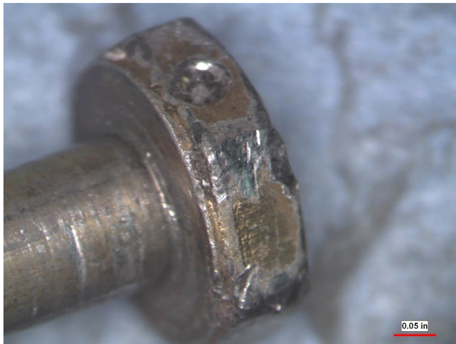
Figure 10. Magnified view showing scratching damage on the head of the AN3H27A bolt. Magnification: x9.
