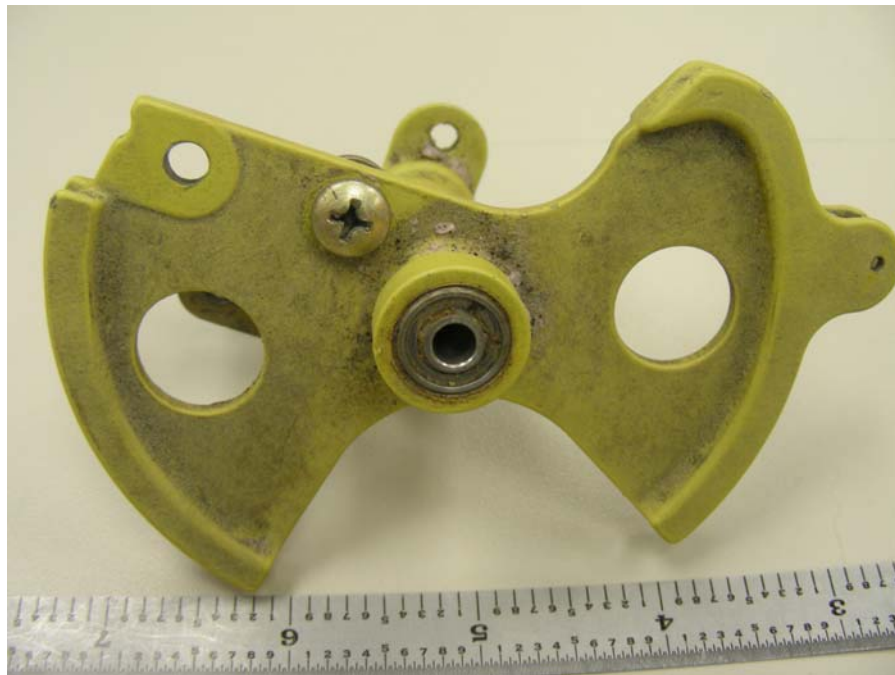
Figure 3. View of the upper surface of the 6260347-12 bellcrank in the condition in which it was received.
