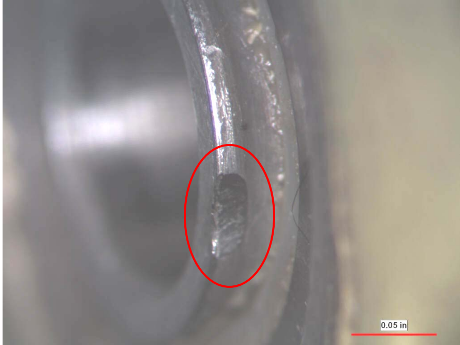
Figure 7. High magnification view of ball insertion groove on the inner race of the lower bellcrank bearing (Figure 6 b). Magnification: x17.3.
