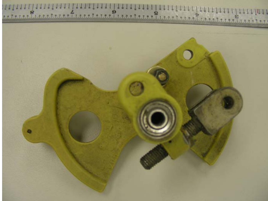
Figure 4 View of the lower surface of the 6260347-12 bellcrank in the condition in which it was received.
