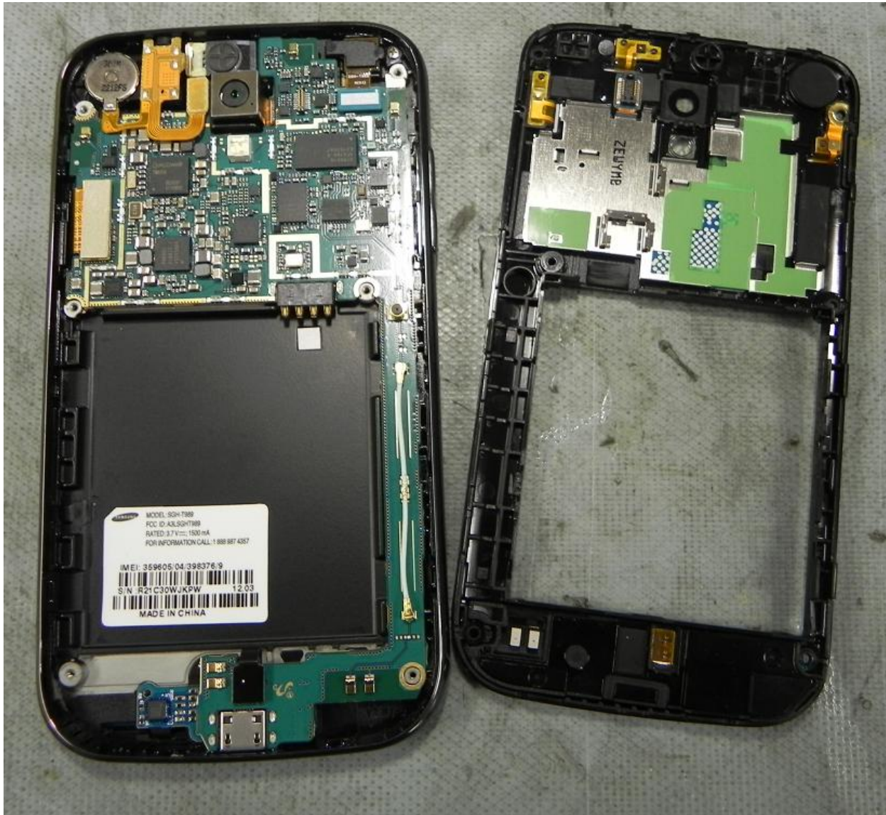
Figure 3. Samsung Galaxy S II – internal inspection.
