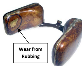
Example: Wear from Rubbing on Large MA Float
