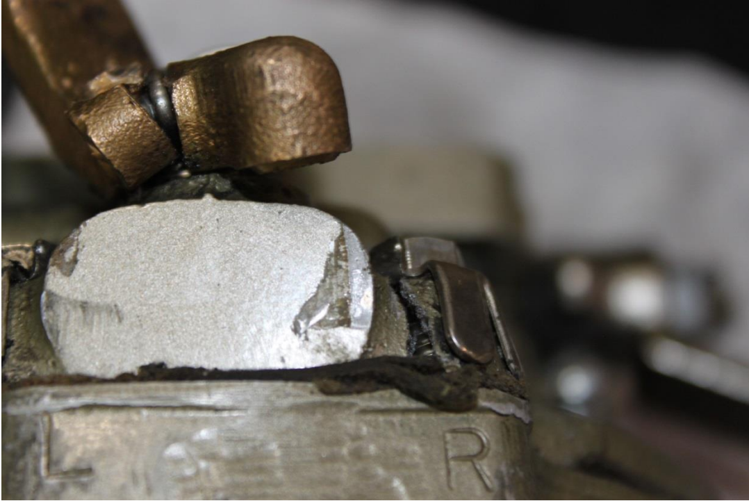
Figure 5: Impact Mark on Boss of Throttle Body Assembly Adjacent to “R” Mark
