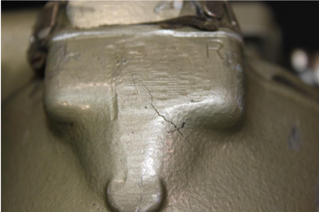
Figure 7: Crack in Carburetor Bowl Assembly
