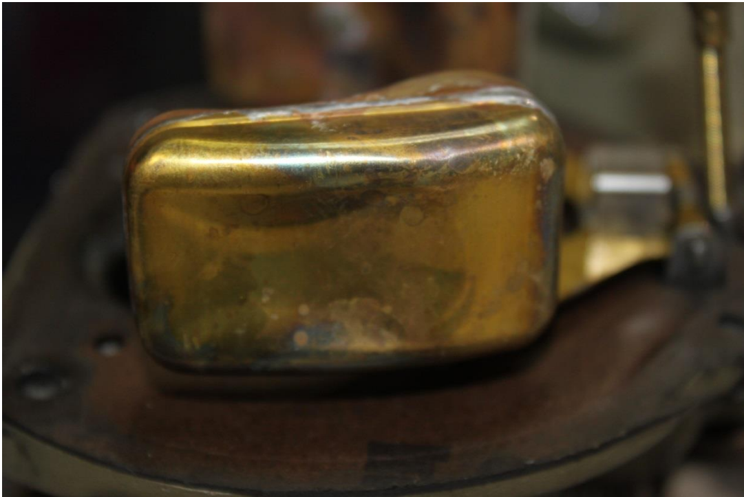
Figure 14: Inward Crush Damage to One of the Pontoons of the Float
