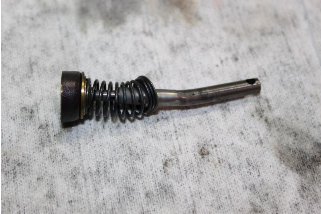
Figure 15: Bent Pump Plunger
