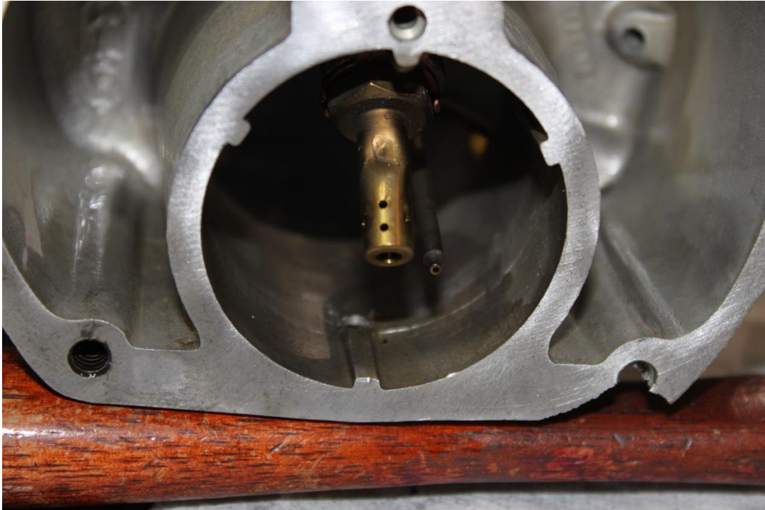
Figure 21: Impact damaged Main Nozzle
