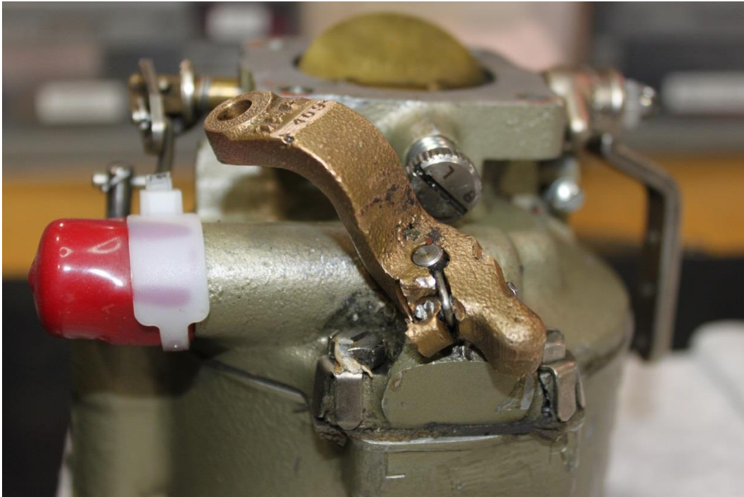
Figure 9: Bent Mixture Control Valve and Mixture Control Lever Assembly.
