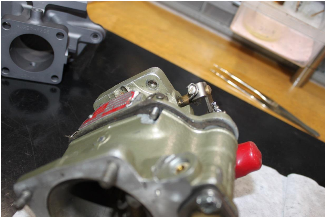
Figure 8: Misalignment of the Throttle Body and Carburetor Bowl Assemblies
