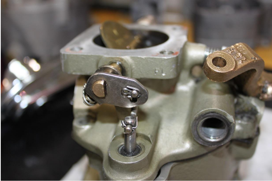
Figure 13: Pump Plunger Connected to Throttle Shaft
