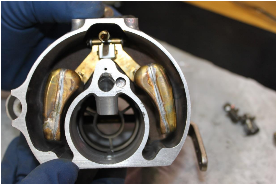
Figure 16: Displaced Pontoon of Float with Cutaway Test Carburetor Bowl Installed
