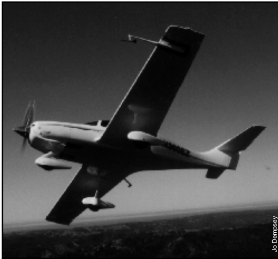
The Express has a cruciform horizontal tail with sweep-back.
