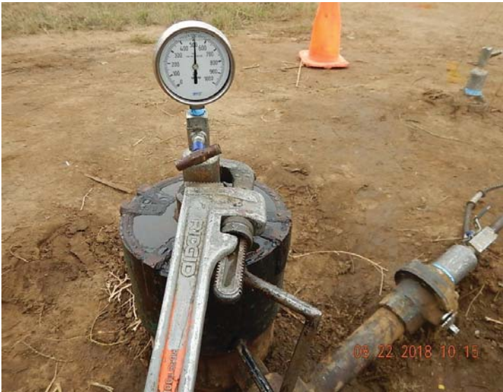
Coors V 6-14Jl pressure test gauge – test Satisfactory
