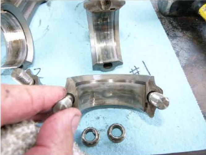
#3 Connecting Rod Part Number: 655911
