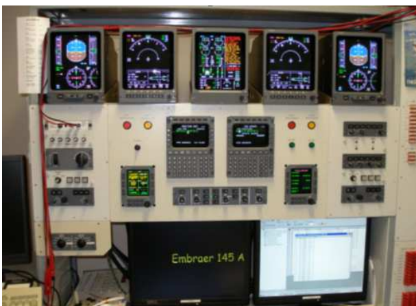
Figure 5. Integration bench for the Primus 1000
