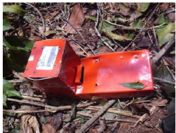
Figure 20: Base of the SSCVR unit, PR-GTD
