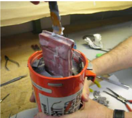
Figure 21: Removal of the memory, PR-GTD SSCVR
