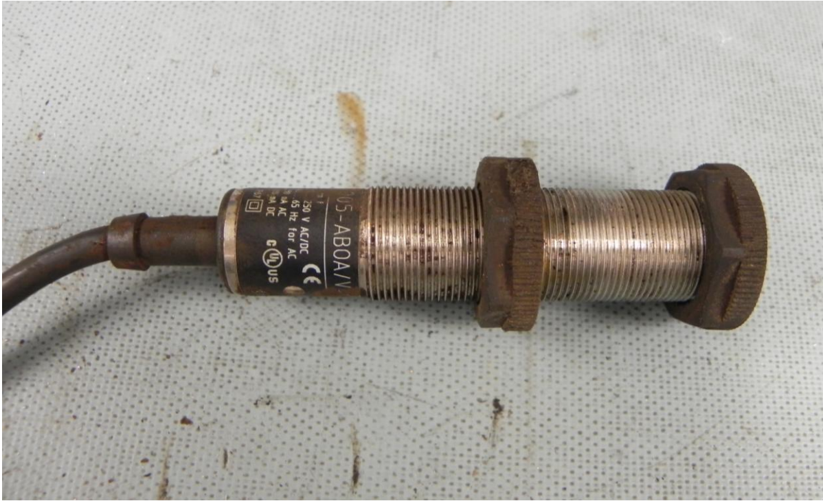
Figure 1. Efactor® model IGO-328 inductive proximity sensor interfaced to the bridge control system and used to verify bridge closure.
