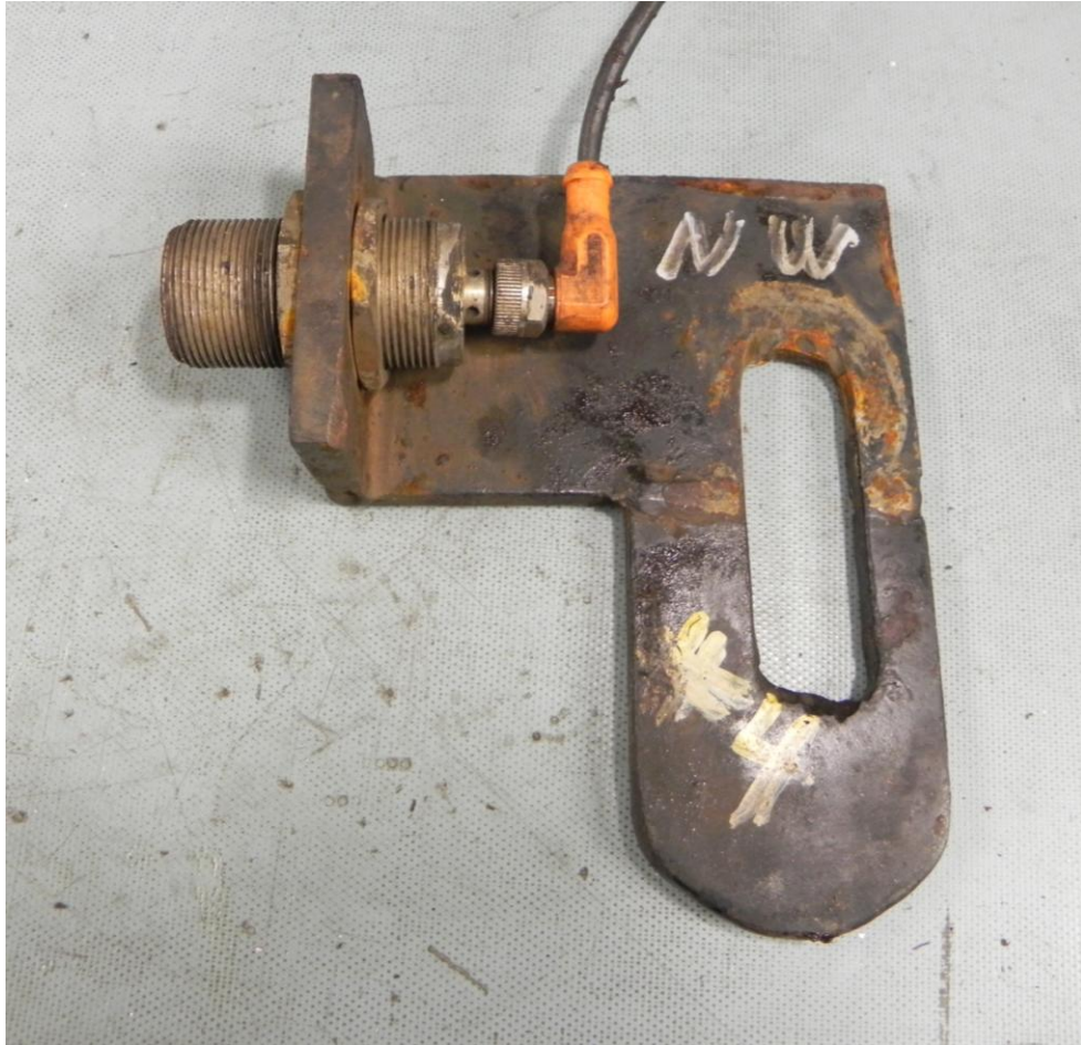
Figure 2. Efactor® model IIM-200 inductive proximity sensor interfaced to the railroad signal system and used to verify rail slide-lock closure.
