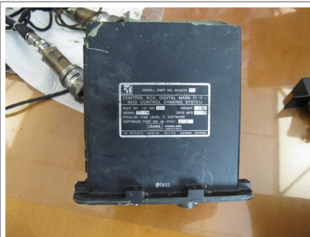
Fig 3 - Control Box (top view)
