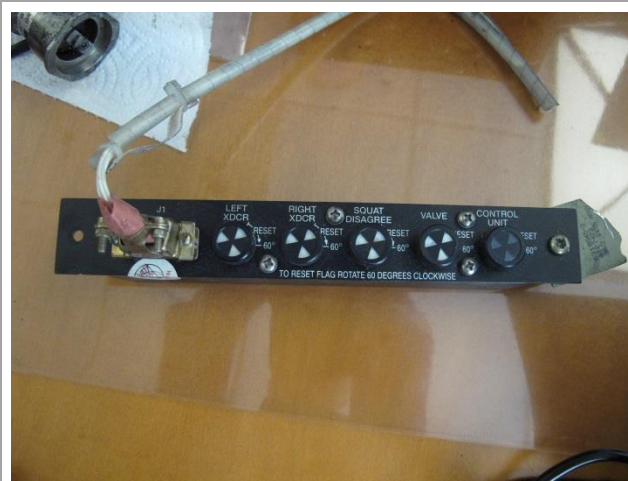
Fig 5 - Skid Control Unit Fault Display - 4/5 flags displayed.
