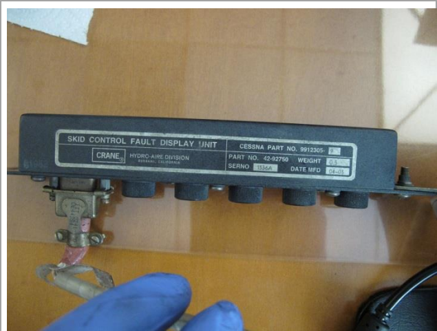
Fig 6 - Skid Control Unit Fault Display (top view).
