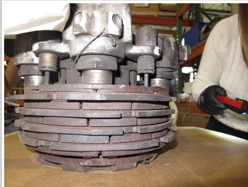
Left brake assembly showing piston extension.
