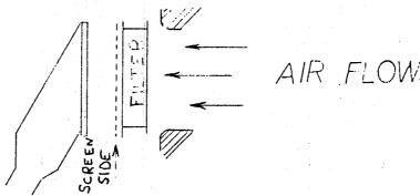
Servicing: Under normal conditions, replace filter element, P/N BA-2405 after 200 hours use or 1 year intervals. Under severely dusty conditions, check daily and replace when element is 50% covered with foreign material.
