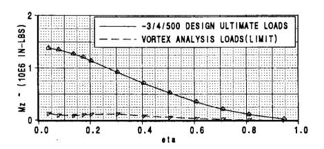
BASED ON WORST CASE POTENTIAL VORTEX VELOCITY PROFILE AT MOST CRITICAL LOCATION ON THE VERTICAL TAIL.
