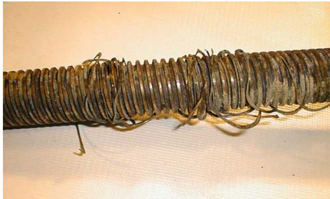
Figure 12. N963AS Jackscrew With Acme-Nut Thread Remnants, Photographed at Recovery Site, 10 February 2000
