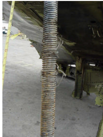
Figure 5. Thread Remnants on Recovered Screw
