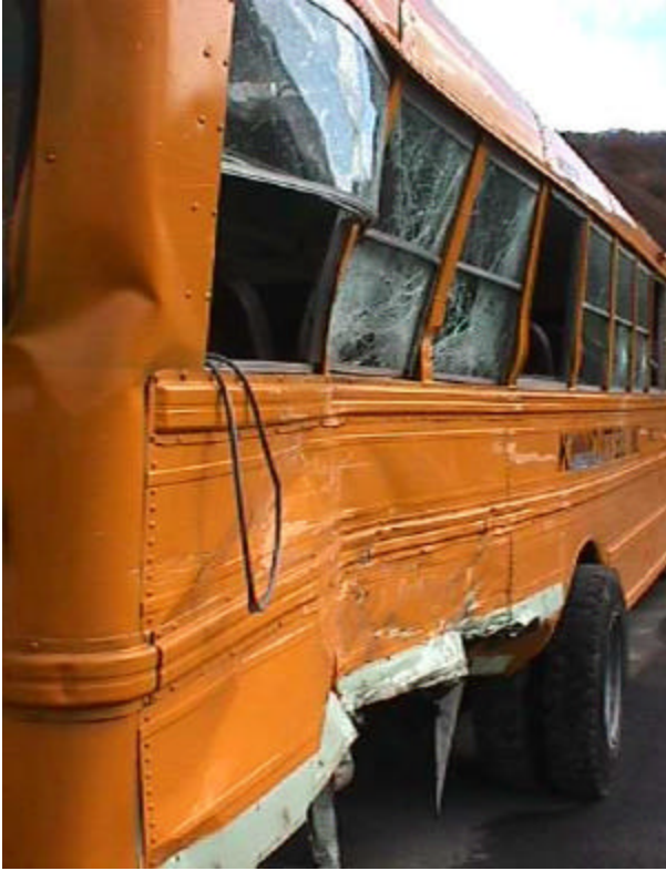
Figure 11: A close-up view of the damage to the bus sidewall on the passenger's side of the bus near the last rows of the bus.
