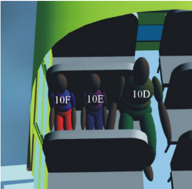
Figure 6: The initial position (a) for the simulated occupant in row 5 on the driver's side of the bus near and the emergency exit door (note orientation of door not to scale) and the initial positions (b) for the simulated occupants in row 10 on the passenger side of the bus.
