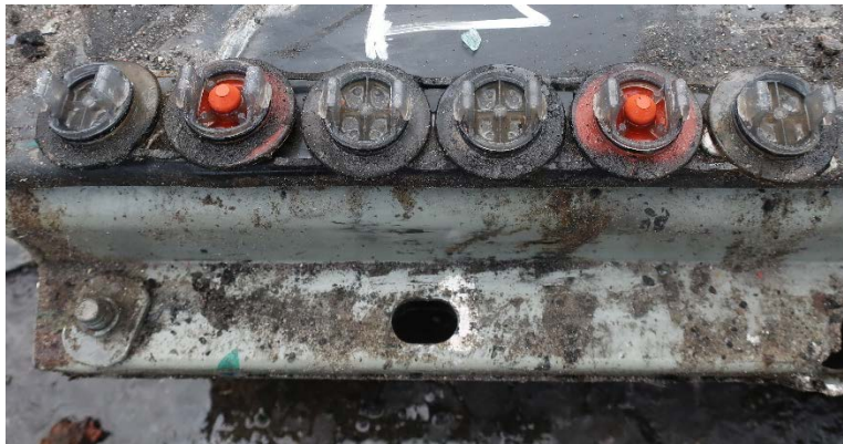
Figure 51. Module 1 valves after removal. Note extensive water on ground which was released during removal.
