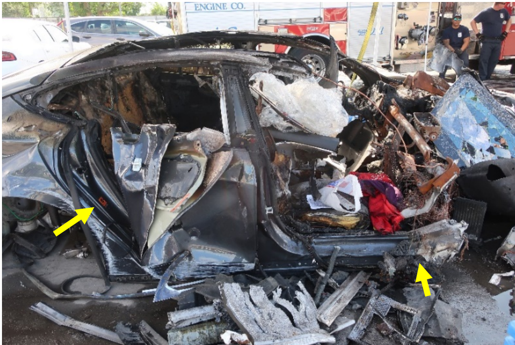
Figure 5. The right side of the vehicle. The added arrow to the left points to a sticker showing a circular saw, described later. The added arrow at the right shows the bend in the passenger door frame.
