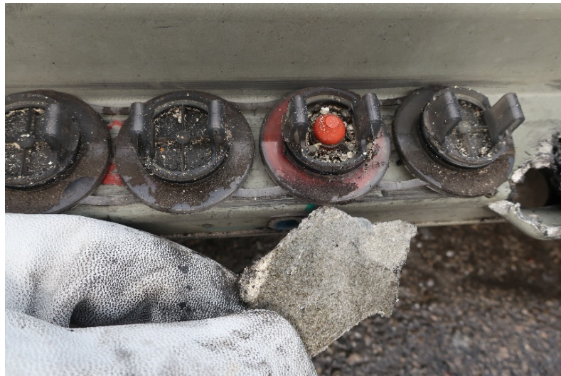
Figure 47. Module 12 valves showing larger grains of tan material and a flake of the mica-like insulation material used above and below each
