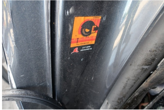
Figure 23. Circular saw sticker in right rear door frame of accident vehicle, as seen in Figure 5.
