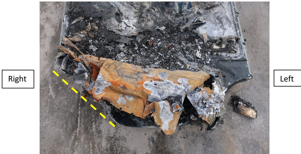
Figure 33. Looking down on the leading edge of the 400 VDC traction battery with forward at the bottom of the photo. Yellow dashed crush line added to photo.
