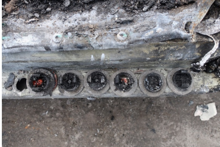
Figure 61. Module 11 valve fire residue contents.
