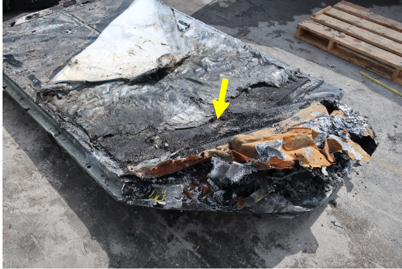
Figure 27. Top of 400 VDC traction battery with arrow to show location of what appeared to be a five inch oblongated hole melted through steel top of the case.
