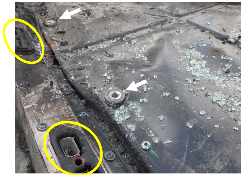
Figure 35. Two mounting bolts along the rear edge of the traction battery are shown at the arrows. (Next Figure shows closer detail of one.) The ovals show the normal battery electrical connections above the battery management system module.
