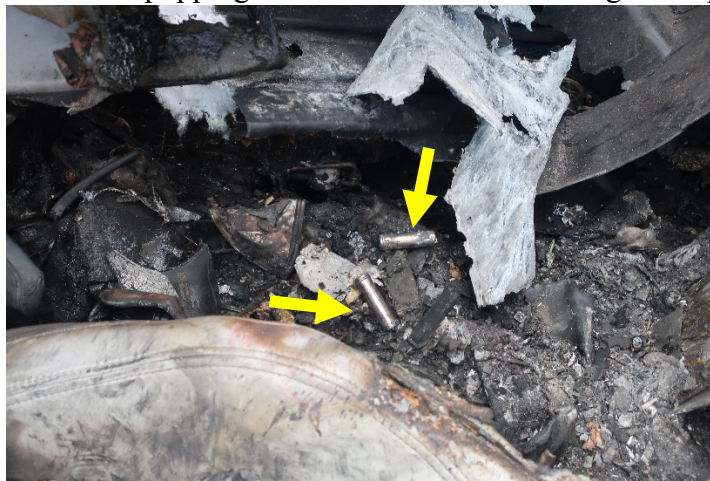
Figure 24. Loose battery cells found under the left front corner of the passenger seat. For orientation, the front of the vehicle is to the right.
