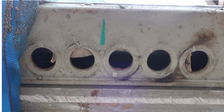
Figure 54. The remnants of internal labels partially block module 5 vent openings.
