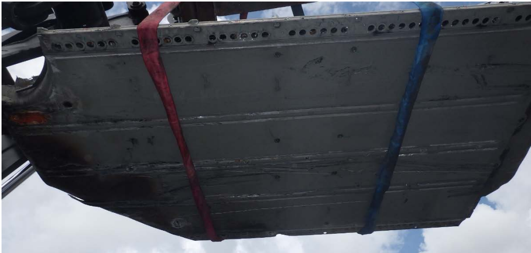
Figure 43. Bottom of the traction battery, as viewed from the left after removal of the rocker covers and vent valves.
