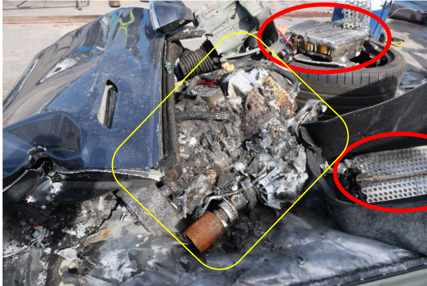
Figure 12. Debris stacked on the 400V traction battery. To the left is the front left door, the traction motor is in the yellow rectangle, and the red ovals surround most of modules 15 and 16. The material under the lower right module was the front trunk liner. 4
