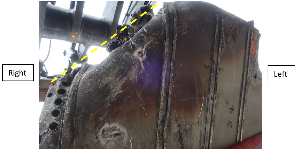
Figure 34. Looking up at the bottom of the 400 VDC traction battery with forward at the top of the photo. Yellow dashed crush line added to photo.
