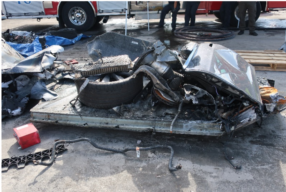
Figure 11. Right side of the 400V traction battery with debris on top. The unburned red item is the 12V systems battery.
