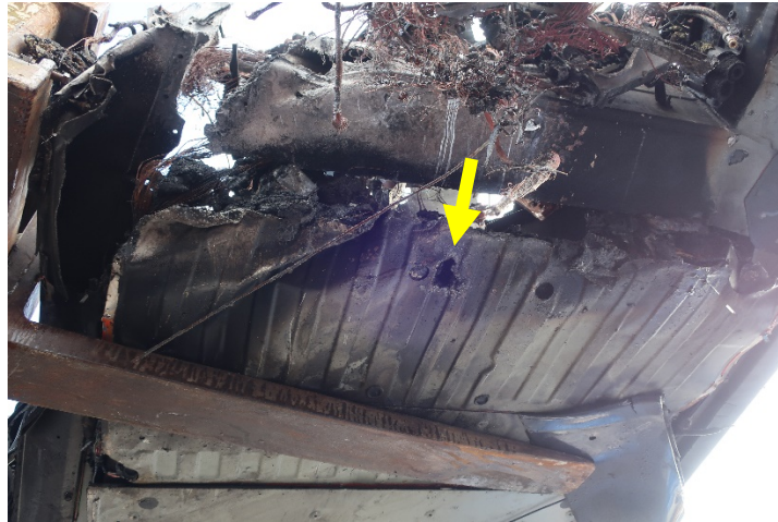
Figure 25. Bottom of passenger cabin, showing hole melted in floor of passenger footwell. For orientation, the bottom of the photo is toward the rear of the vehicle.
