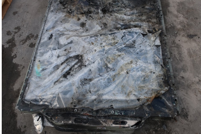
Figure 38. Intact insulation and plastic water liner layers covering rear portion of 400 VDC traction battery.
