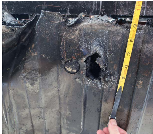
Figure 26. Closer view with scale shows the hole was about three inches in longest dimension.
