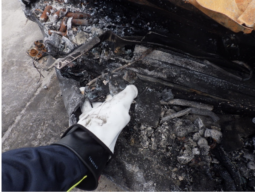
Figure 42. Remnants of the pyrotechnic fuse.
