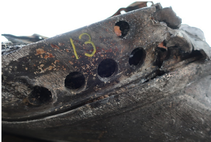
Figure 63. Module 13 vent openings.
