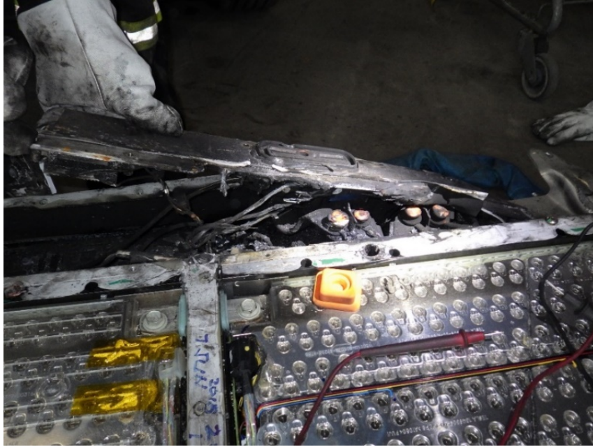
Figure 76. The burned interior of the BMS contrasted with the intact nature of modules 1 and 2.
