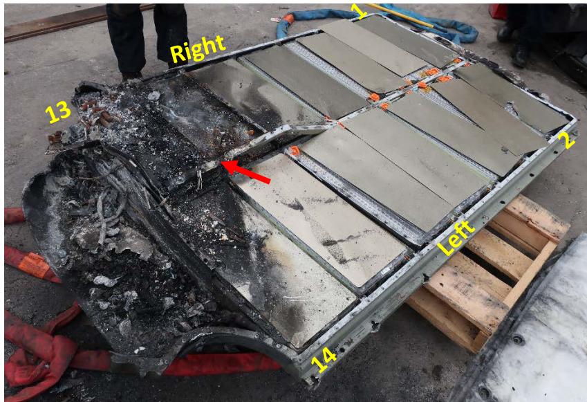
Figure 66. Mica-like sheets cover the individual modules. 13 Numbers have been added to denote modules. The red arrow points to the area of the missing module 11 terminal which was beneath the set of holes.
