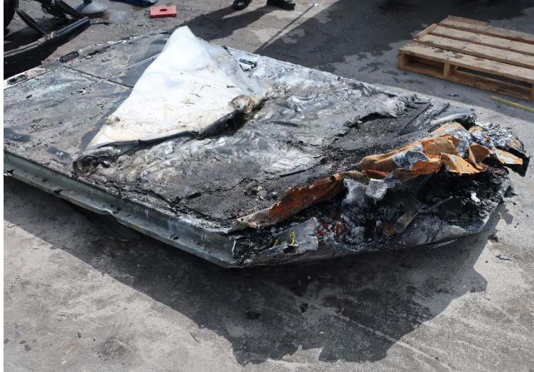
Figure 32. Twist in battery with forward right higher than the aft left.
