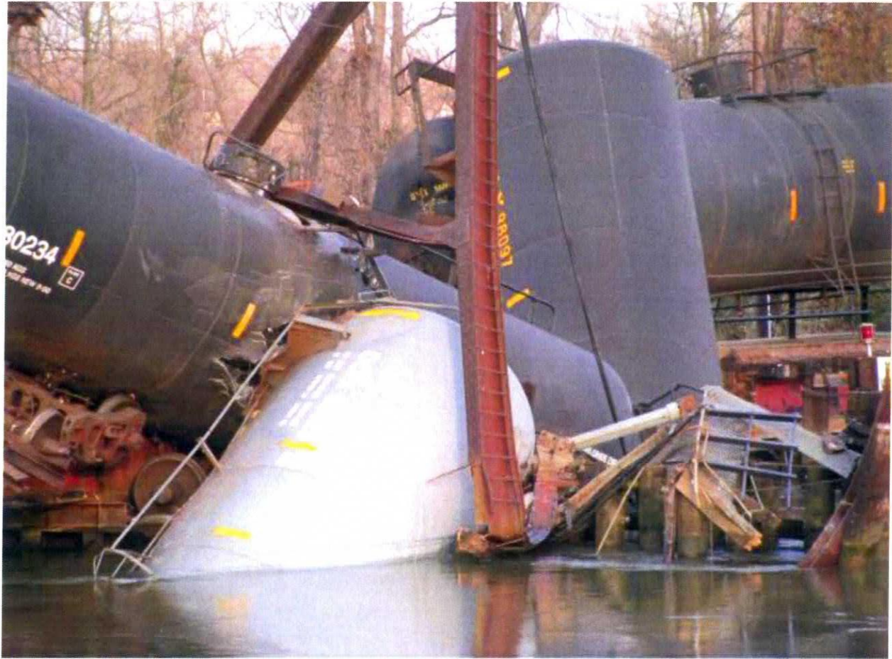
Figure 4: Photograph of tank car OCPX 80323 and the breach in tank car OCPX 80234
