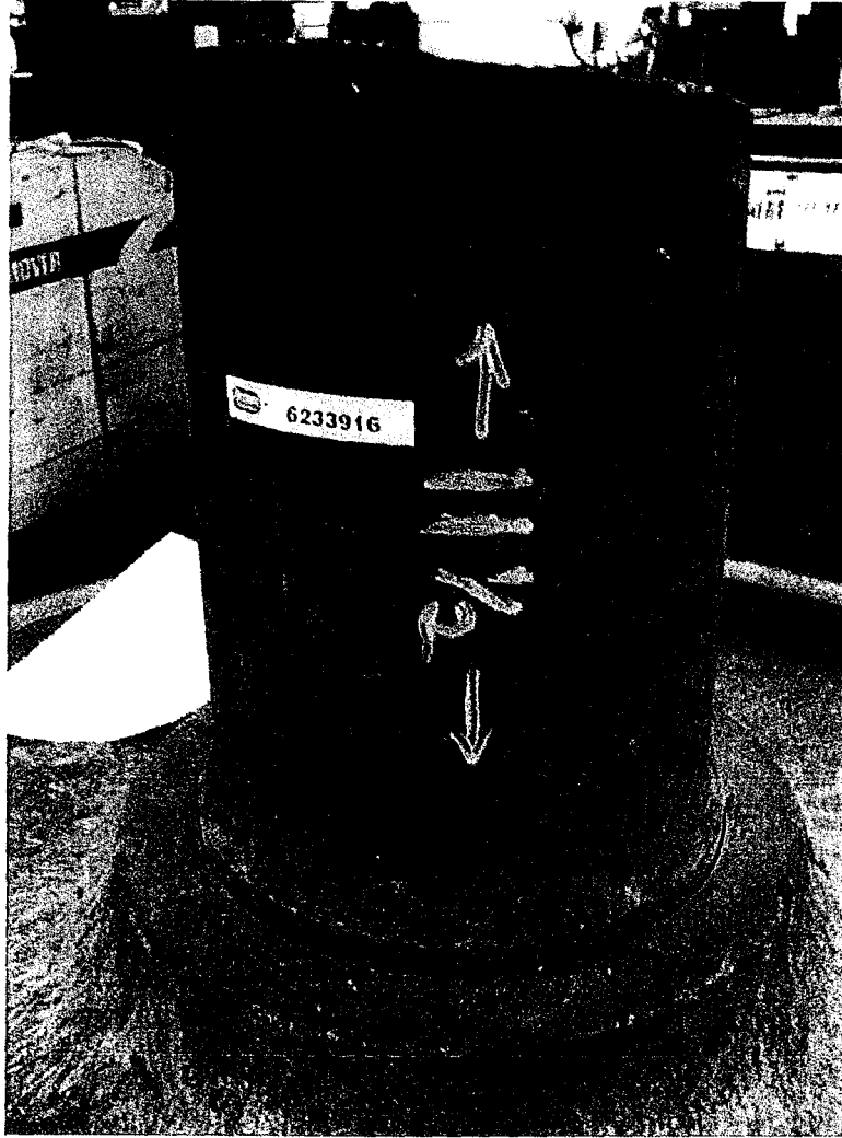
Photograph 2: The R3 side of the broken axle as received at the Laboratory.
