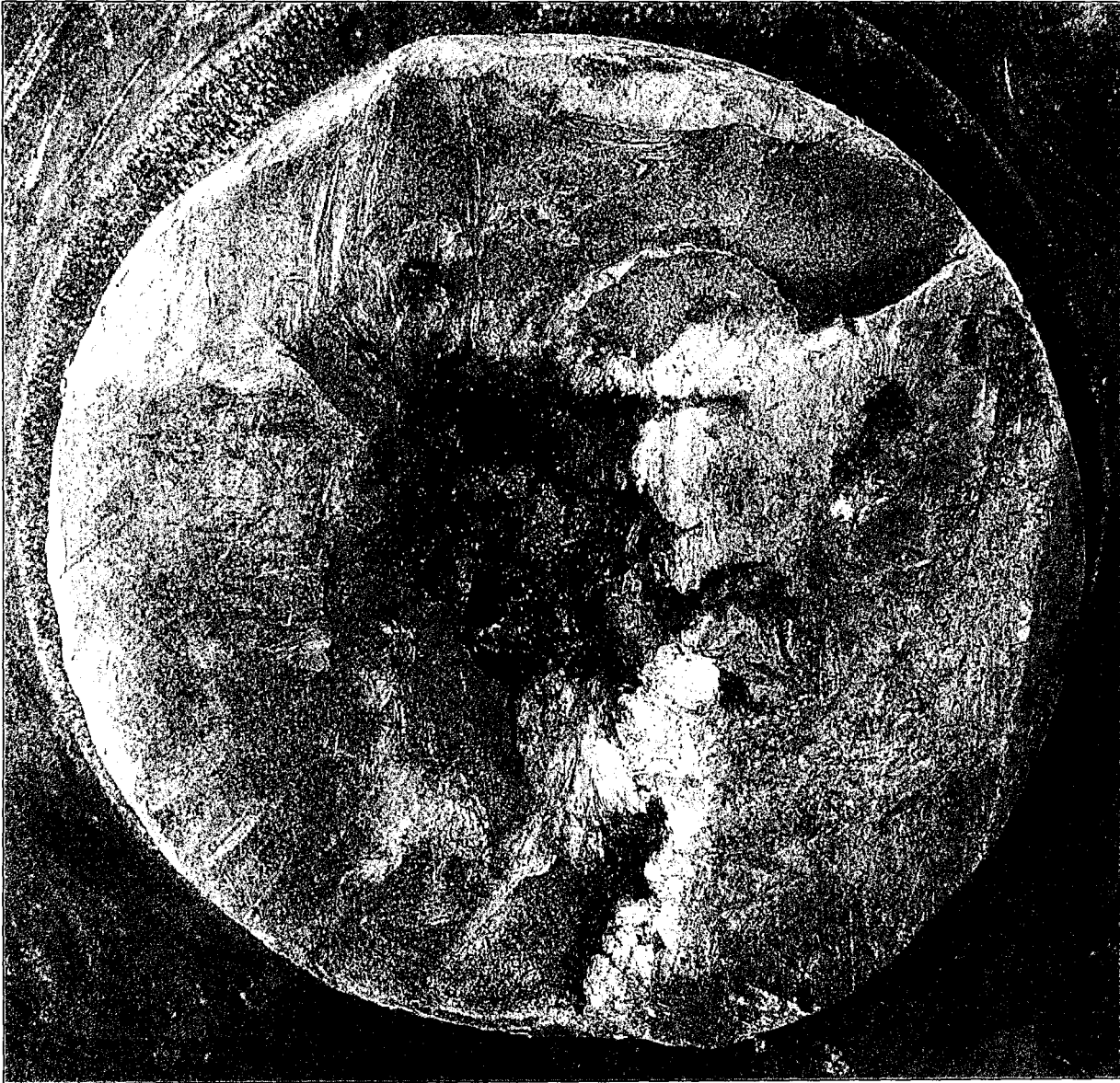
Figure 4: Fracture face view taken from the short axle end.
